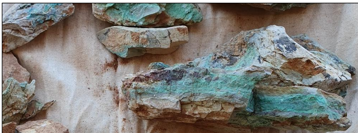
Photo 1. Rock chip sample KB03113, which returned 15.3% Copper 1 , comprised of oxidized white meta-tuffaceous siltstone with oxide copper mineralisation (green in photo).
