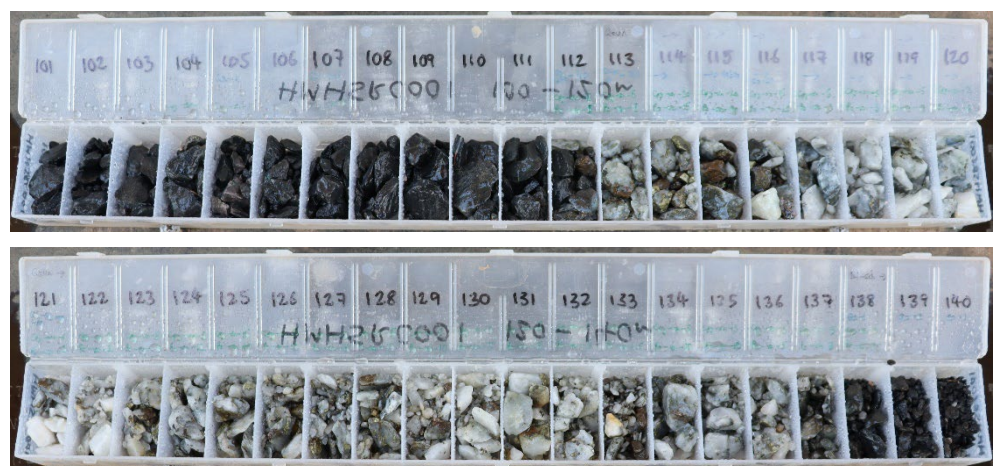
Figure 1. Chip Trays HMHSRC010, 100-140m. 14m at 3.34% Cu and 0.72g/t Au from 113m is located within a clean quartz vein zone.
