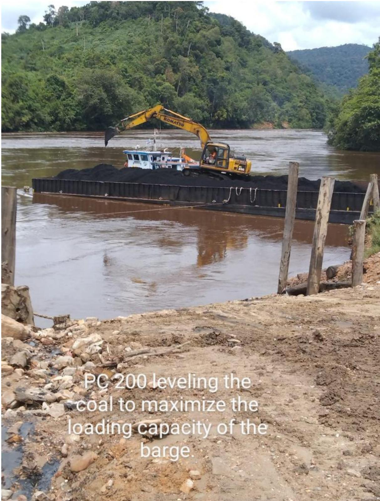
PC 200 leveling the coal to maximize the loading capacity of the barge.
