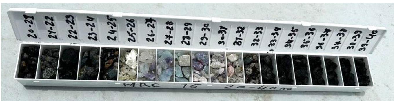
Figure 2: Chip-tray of 20m-40m interval of MRC15.
