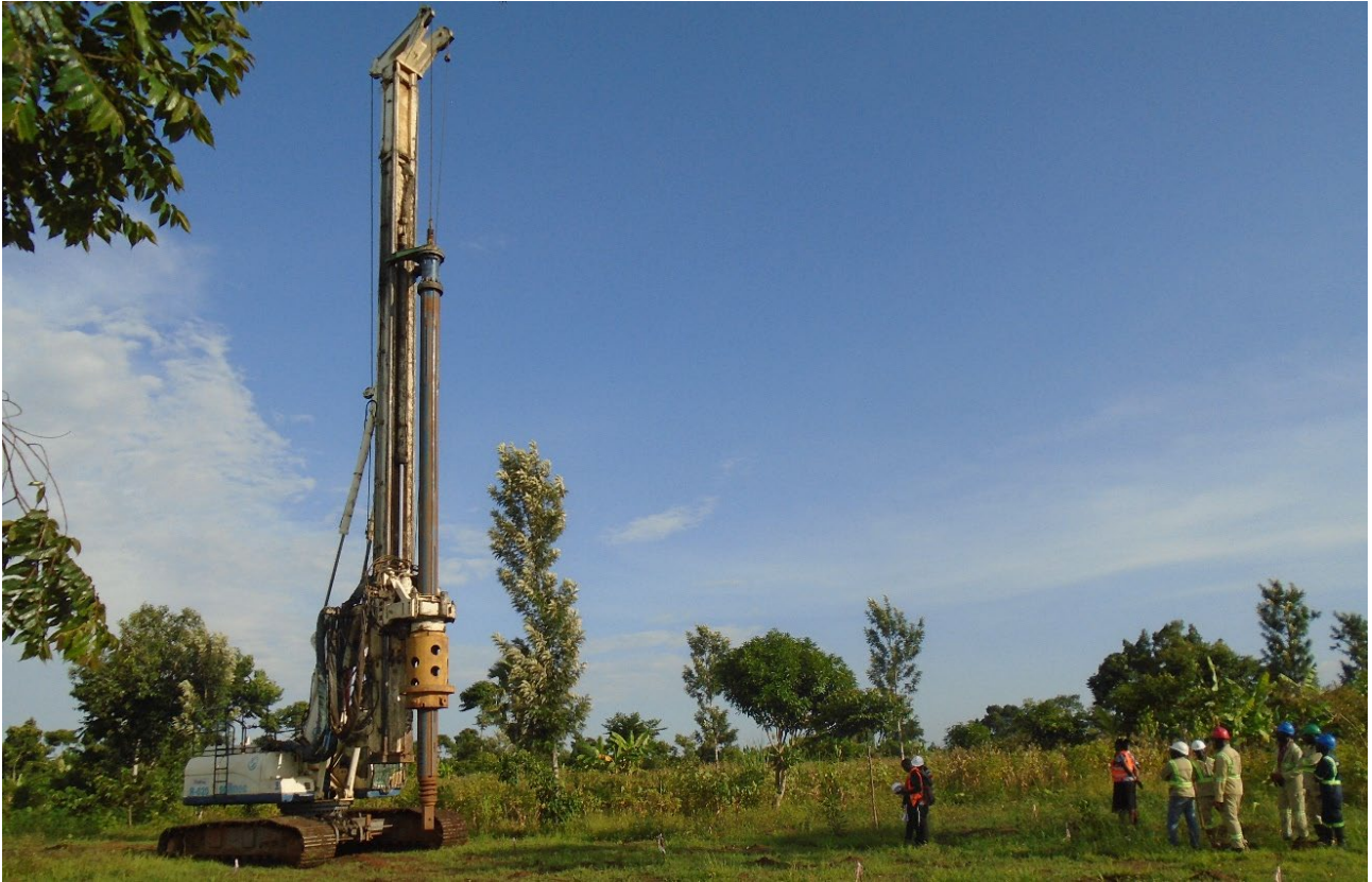
Figure 4: Auger drill mobilised to test site to collect bulk sample test material.
