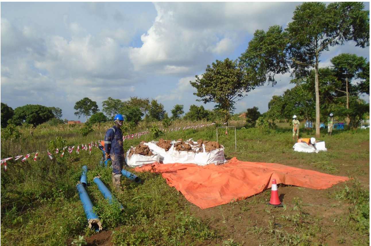
Figure 5: Bulk sample being collected for desorption column and crib metallurgical test work program.
