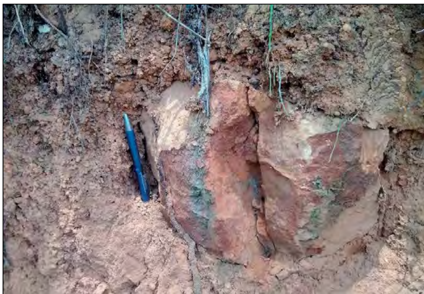
Figure 34: Monazite rich corestone exposed during excavation of drill access road Source: CSA Global 2023
