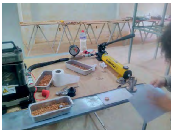
Figure 10. Vacuum apparatus and preparation of compressed clay discs for XRF analysis. The pellet may be noted on the sheet of paper and is the correct size for use in the hands free XRF unit used.
