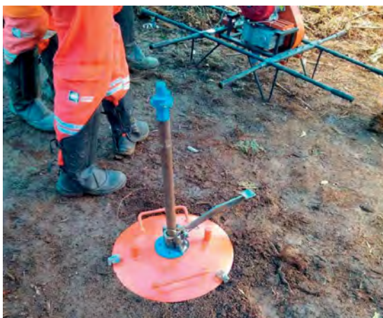
Figure 2. Auger site set up with bubble levelled metal collar protector in place. This is positioned after first meter completed (A horizon/organic material). Foot hold allows drilling down to 30 m.
