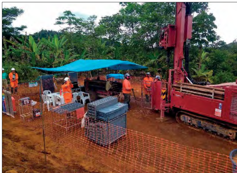
Figure 13. Sonic drill rig in operation Source: CSA 2023
