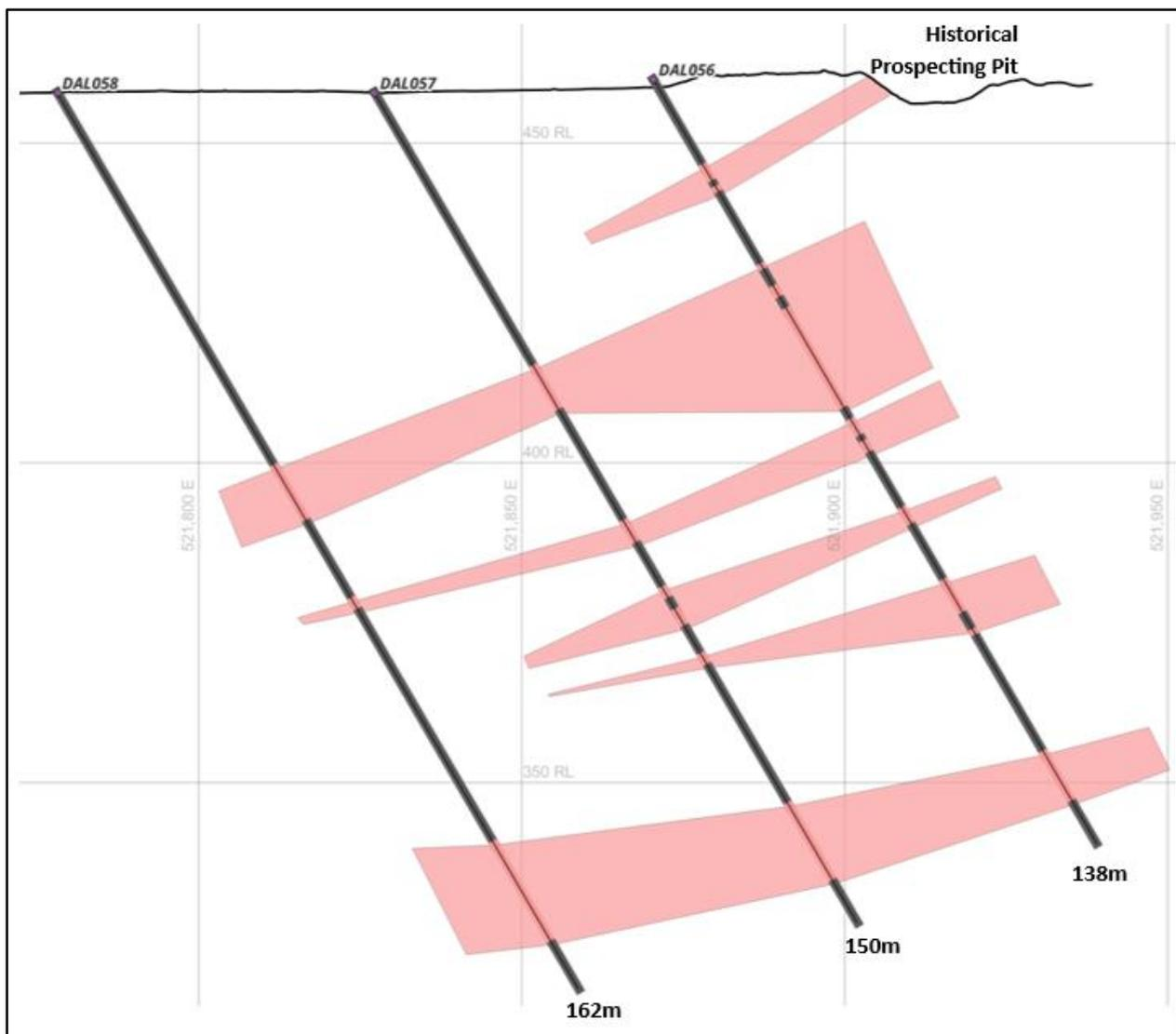
**Figure 3:** Schematic cross-section over the northern drill line showing pegmatite distribution and continuity.
