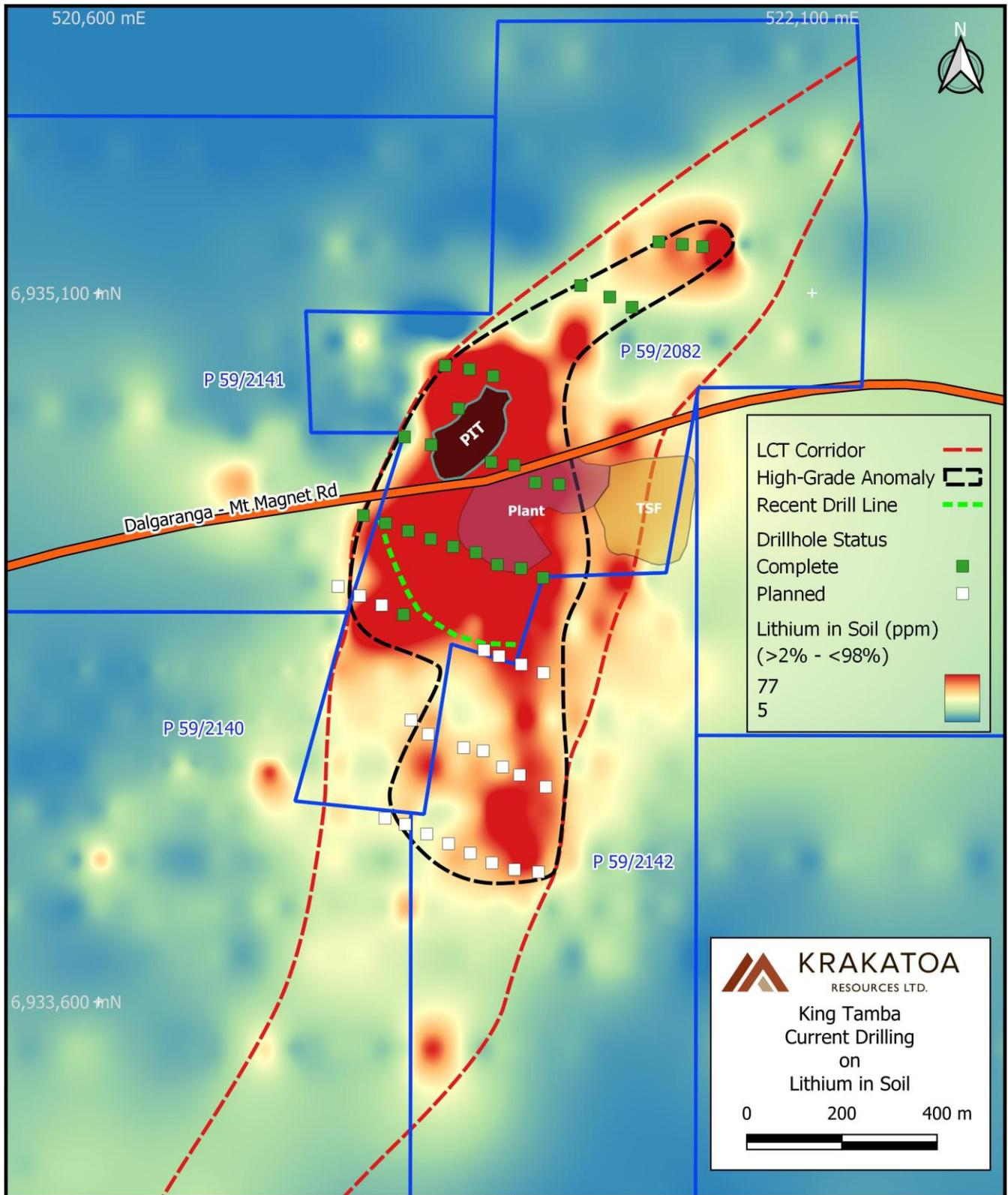
**Figure 2** Drill Collar Locations shown in relation to the high-grade lithium soil anomaly (red high, blue low) of interest.
