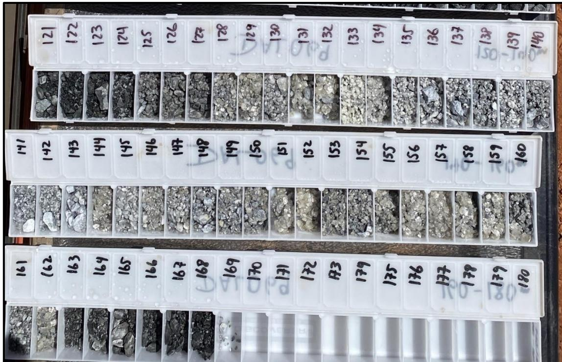
**Figure 1** Photograph of drill hole DAL069 chip tray showing 39m intersection of pegmatite
