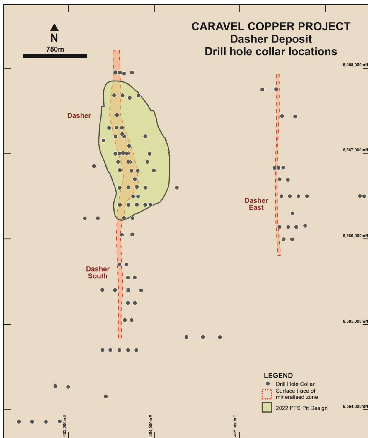
Figure 10: Plan map of drilling and surface expression of mineralisation at Dasher with 2022 PFS pits
