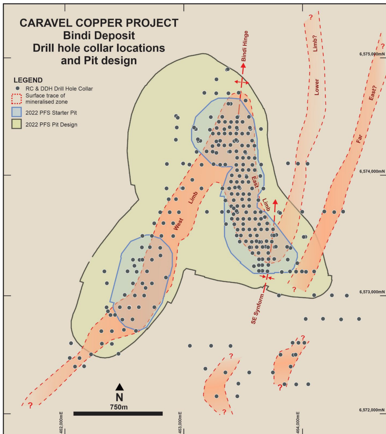
Figure 5: Plan map of drilling and surface expression of mineralisation at Bindi with 2022 PFS pits
