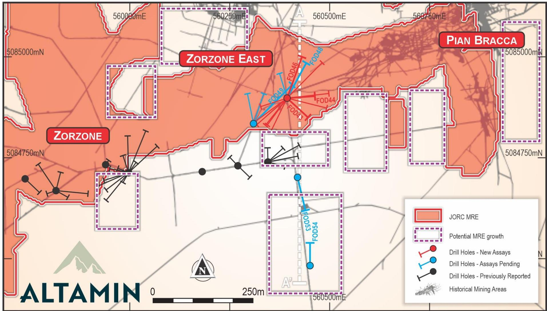
Figure 2: Plan detail showing reported drill holes & section line at central Forcella level (940m RL)
