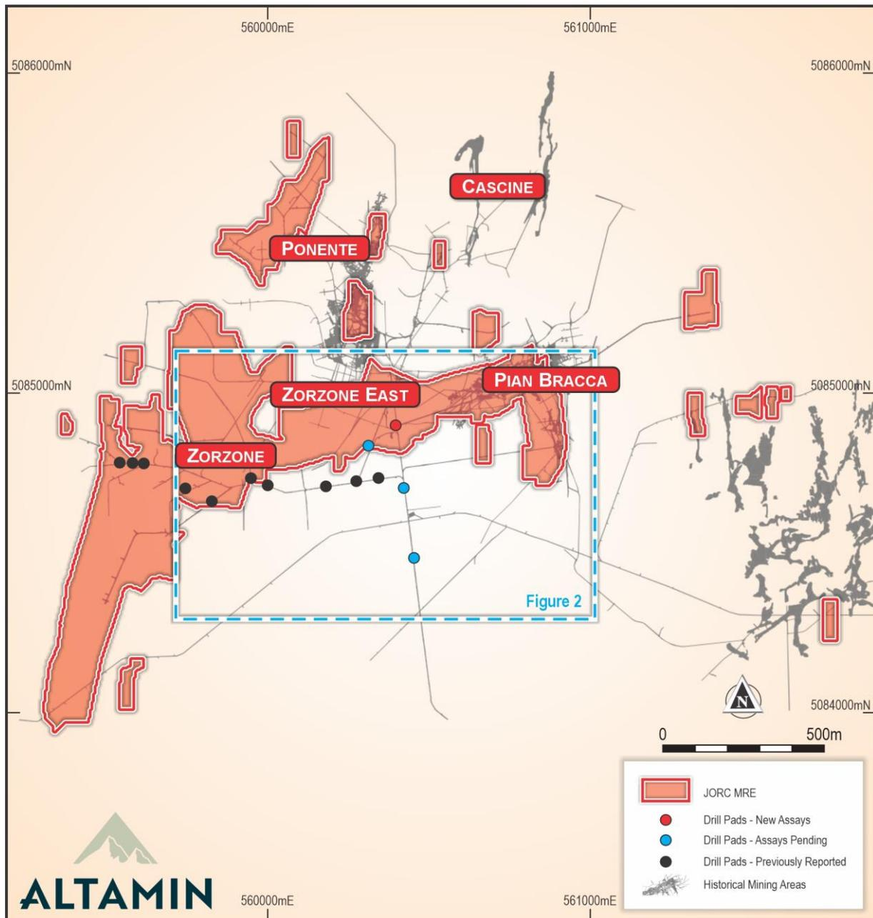
Figure 1: Plan overview showing the Mineral Resource Estimate footprint, location of reported drillholes & previously reported drill pads from this campaign
