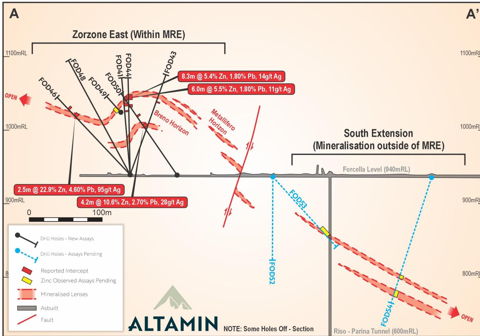
Figure 3: Vertical section A-A' looking west showing interpreted mineralisation & drilling intercepts
