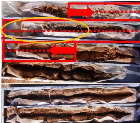
Some of the highest grades of uranium mineralisation in single 1-2 m lens around a large clay pan within the dunes that sit at the back of the lunette shaped Millipede orebody.
