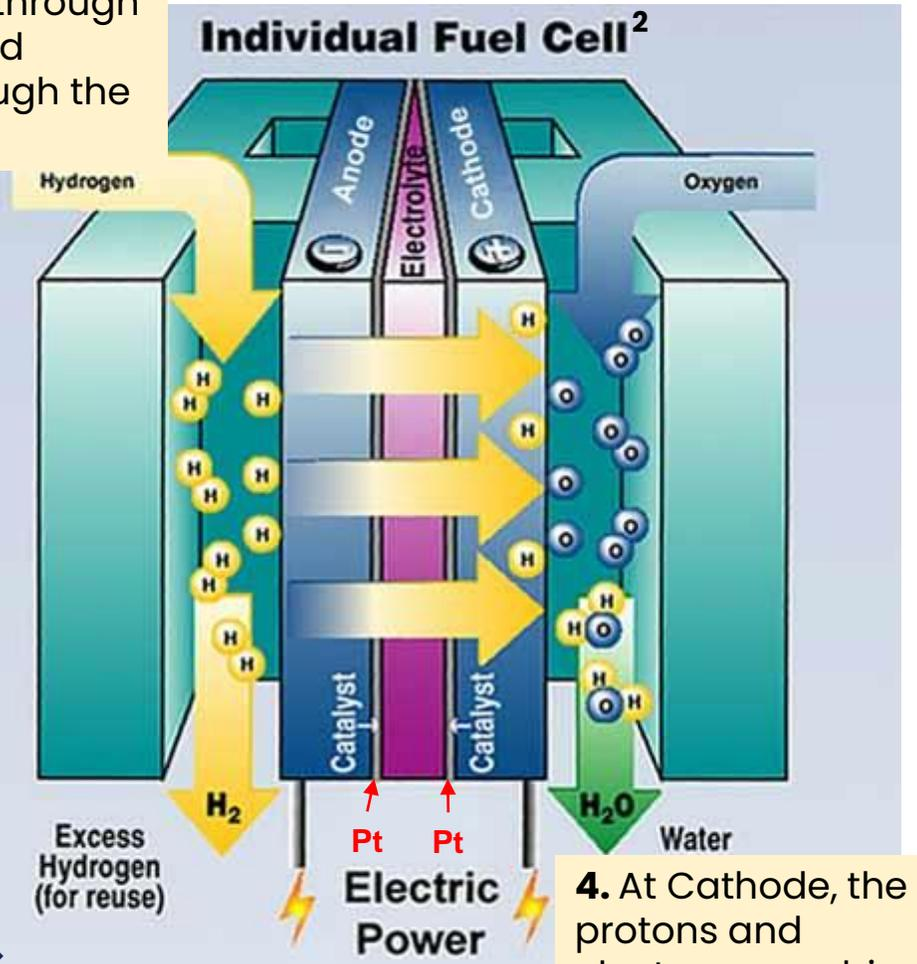
4. At Cathode, the protons and electrons combine to create water as waste
