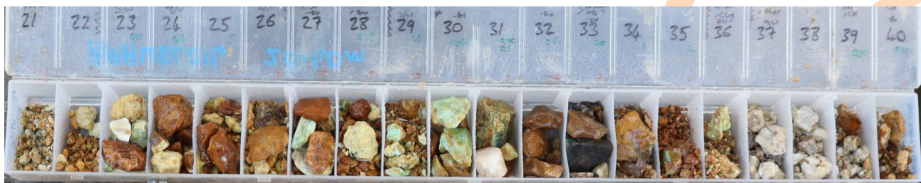
Figure 1. Copper oxide visible in drill chips from HMHWRC0014 (20-40m). A copper grade of 2.78% was reported between 31m and 36m (see ASX Announcement 31 October 2023).
