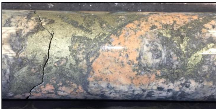
**Figure 4.** Breccia-hosted copper mineralisation west of the Corvette deposit, comprising 5.8 metres at 1.97% Cu & 179ppm Mo (photograph from ~170 metres down hole in 23MYDD434, core diameter 45mm, ASX MAG 6 December 2023).
