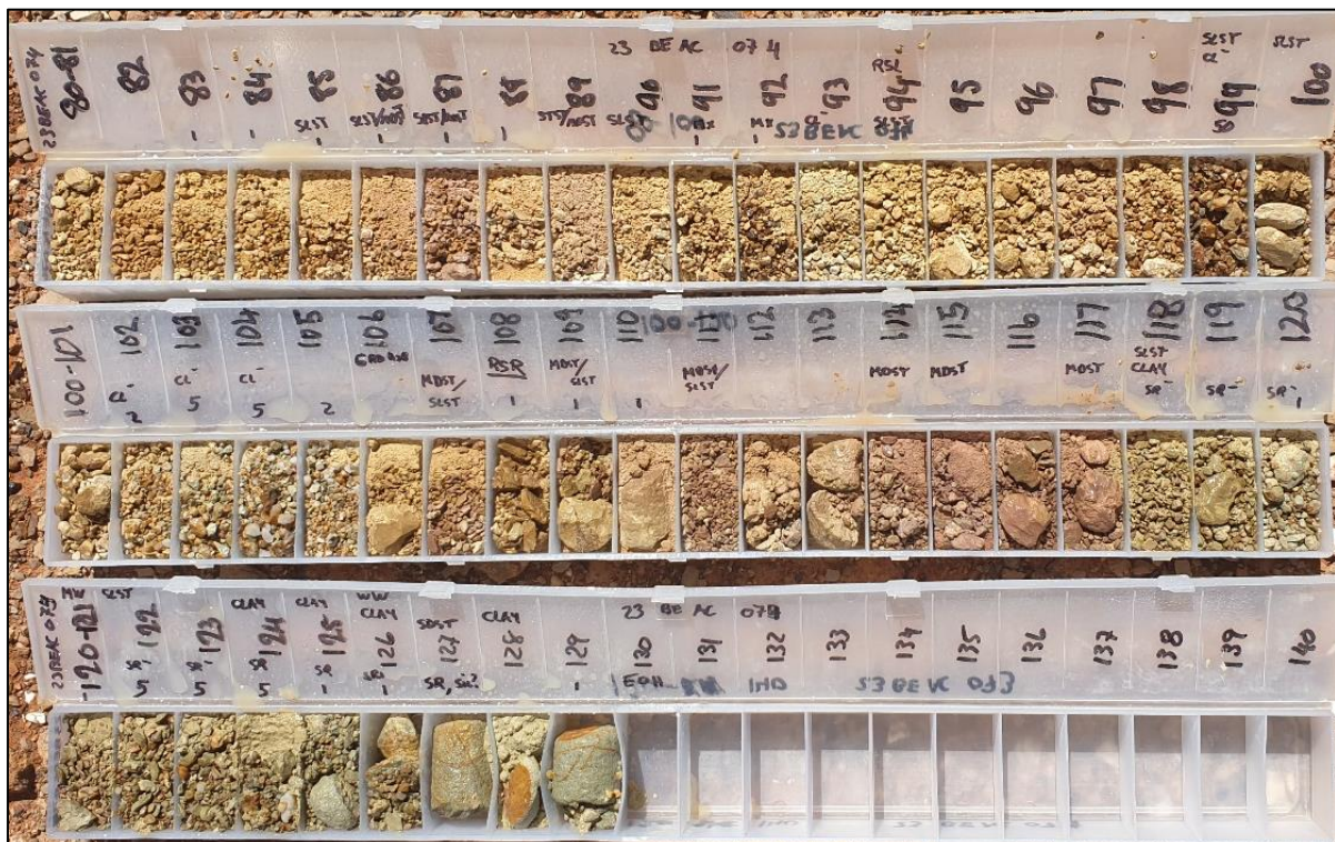
Photo 2. Chip trays from deepest portion of hole 23BEAC074, showing Lower Saprolite (RSL) and Saprock (RSR) boundaries, with Silica alteration (SR = Sericite) towards the bottom of hole.
