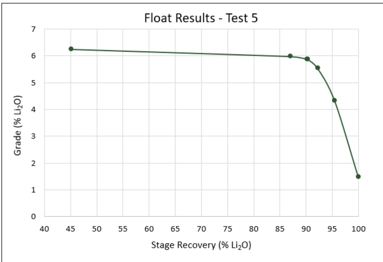
**Figure 6 - WOO Fines Flotation grade / recovery stage results**
