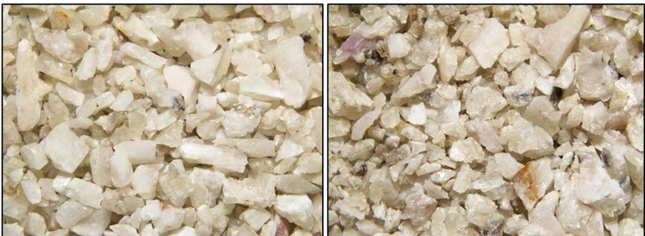
**Figure 4 - HLS concentrate fractions grading ~6.0% Li<sub>2</sub>O (left) and ~5.5% Li<sub>2</sub>O (right)**
