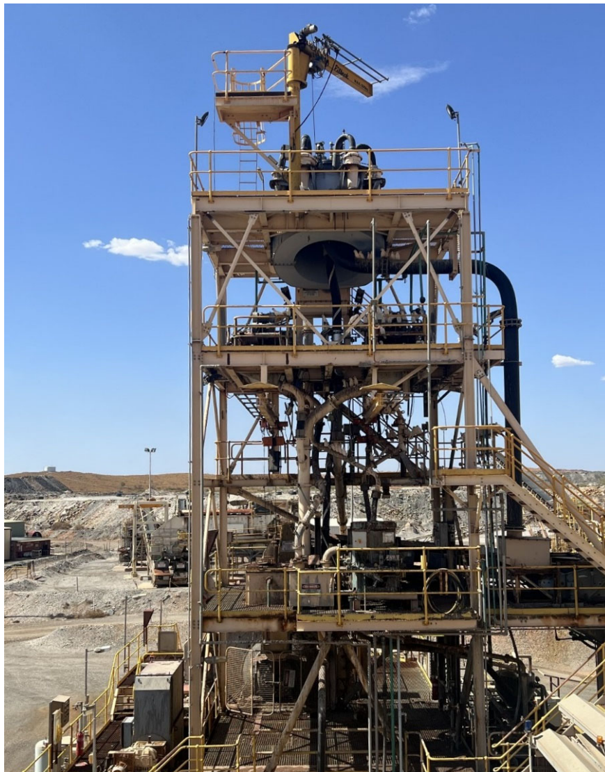
Figure 11: Deep cleaning the crushing/screening circuit and cyclone tower will commence in February 2024. Pipework will be inspected and/or replaced.
