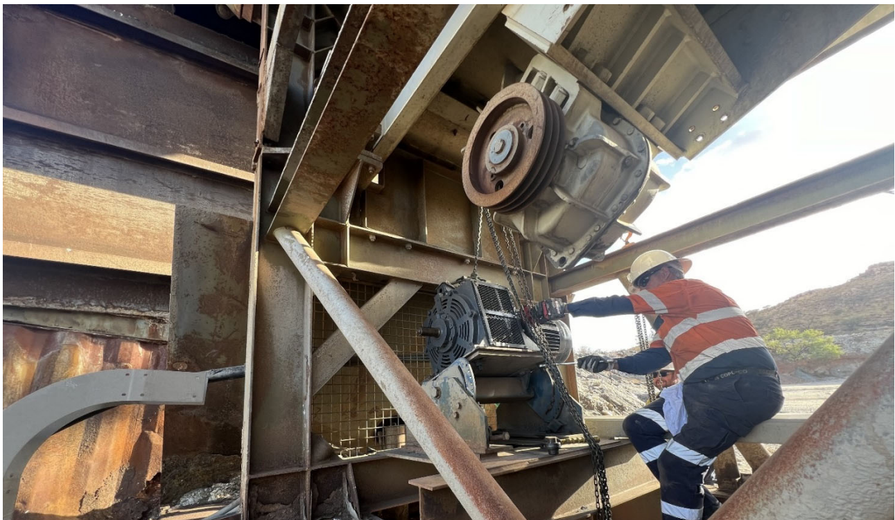
Figure 1: Black Cat maintenance team replacing primary crusher pan feeder motor.
