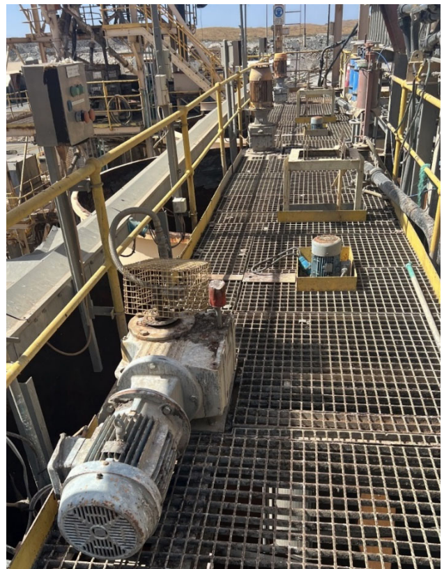
Figure 9: CIL agitator motors and gearboxes to be stripped and serviced with only one motor and gearbox requiring replacement.
