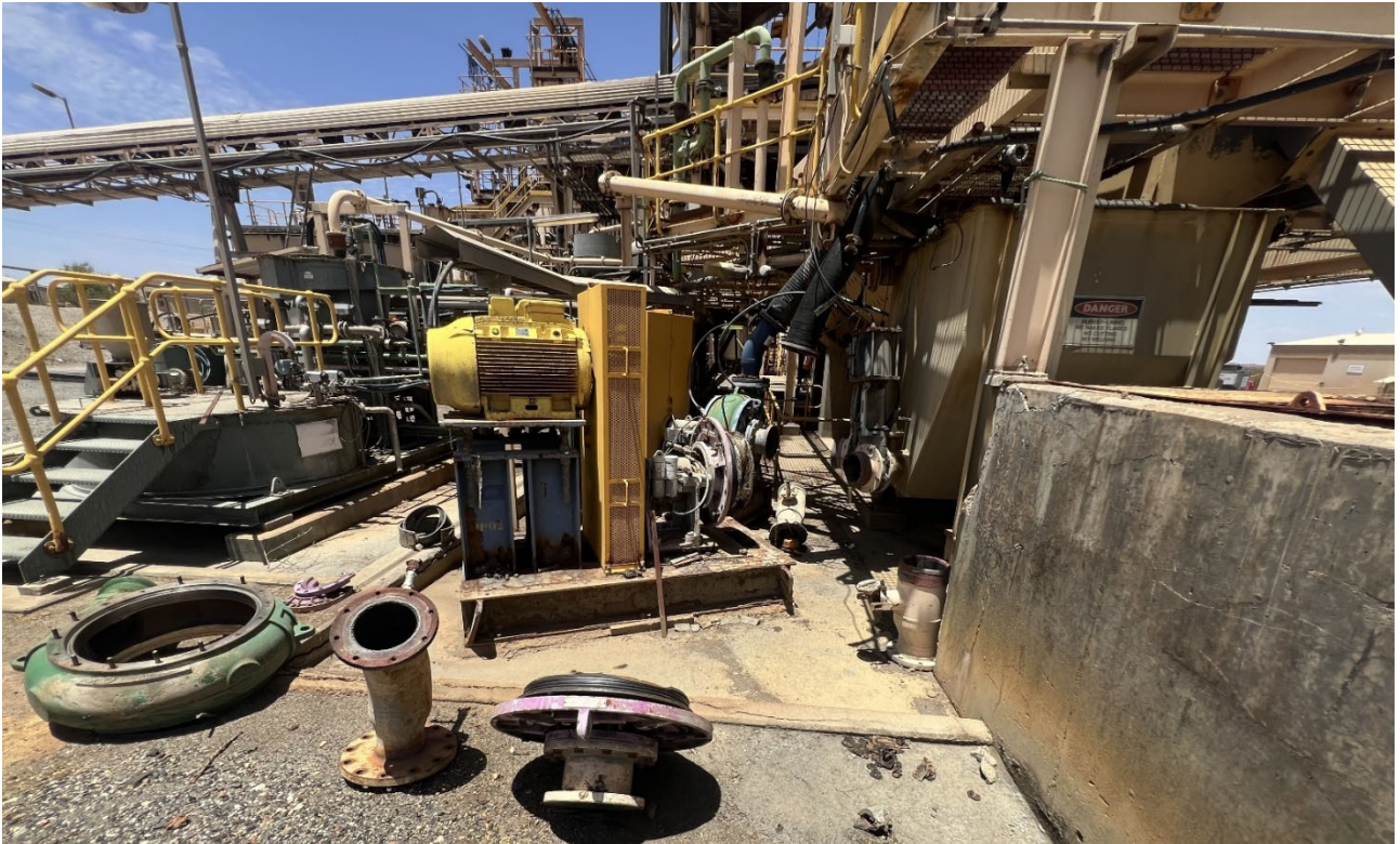
Figure 10: Cyclone feed pump that is stripped and ready for servicing. All sump pumps within the gravity/leach areas are operational. Servicing of pumps will continue during the March 2024 quarter.
