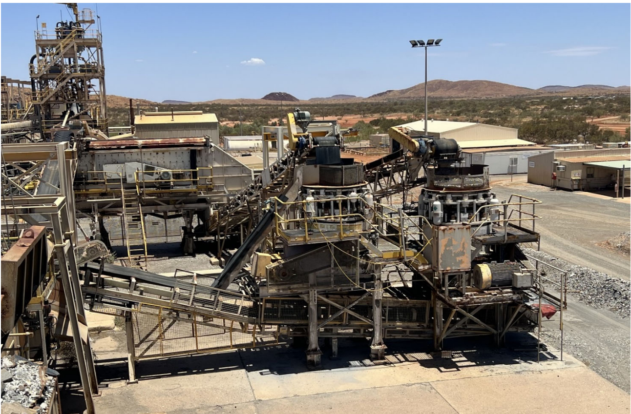
Figure 6: Secondary (left) & tertiary (right) cone crushers are operable.
