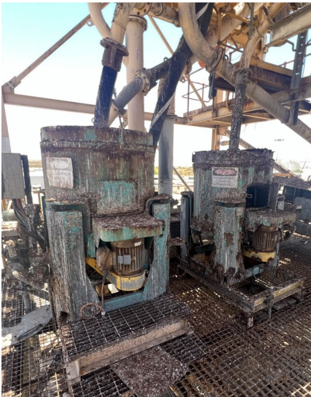
Figure 8: Existing Knelson gravity concentrators that will be removed, stripped for spares and replaced with new units, in the process of ordering.
