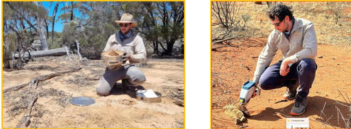
Figure 1 - Asra's field team soil sampling and using handheld pXRF machine at Kookynie West.
