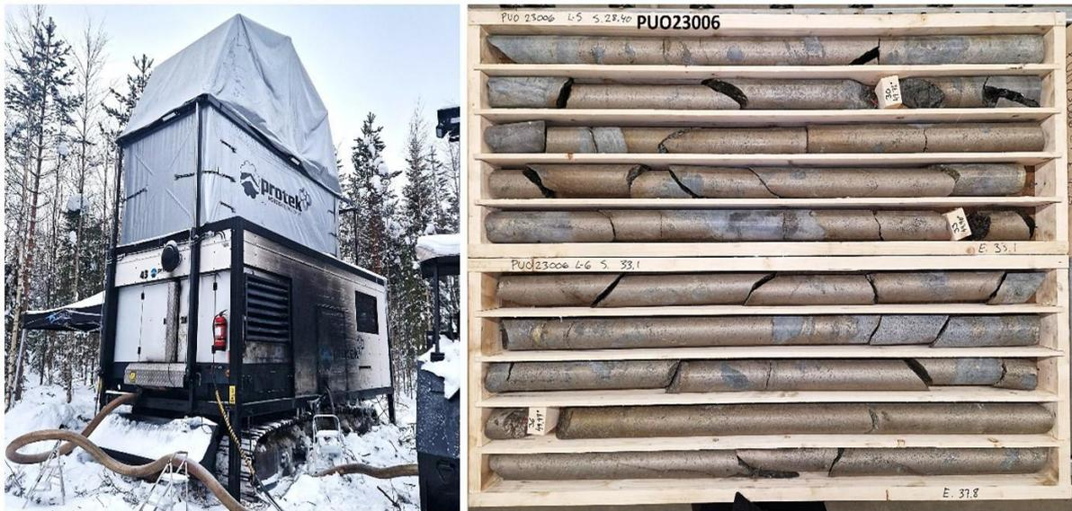
**Figure 7:** Drilling rig on-site at Puolalaki and massive sulphide mineralisation in drillhole PUO23006, (28.4-37.8m).
