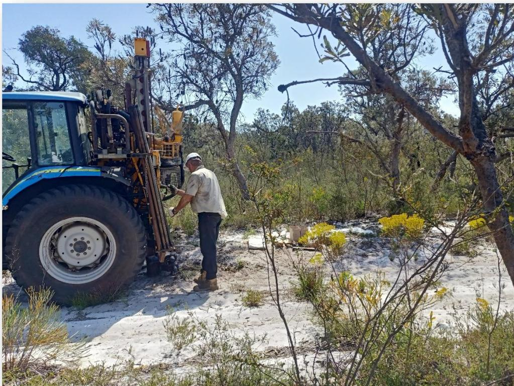
*Figure 4: Vacuum drilling at Muchea*
