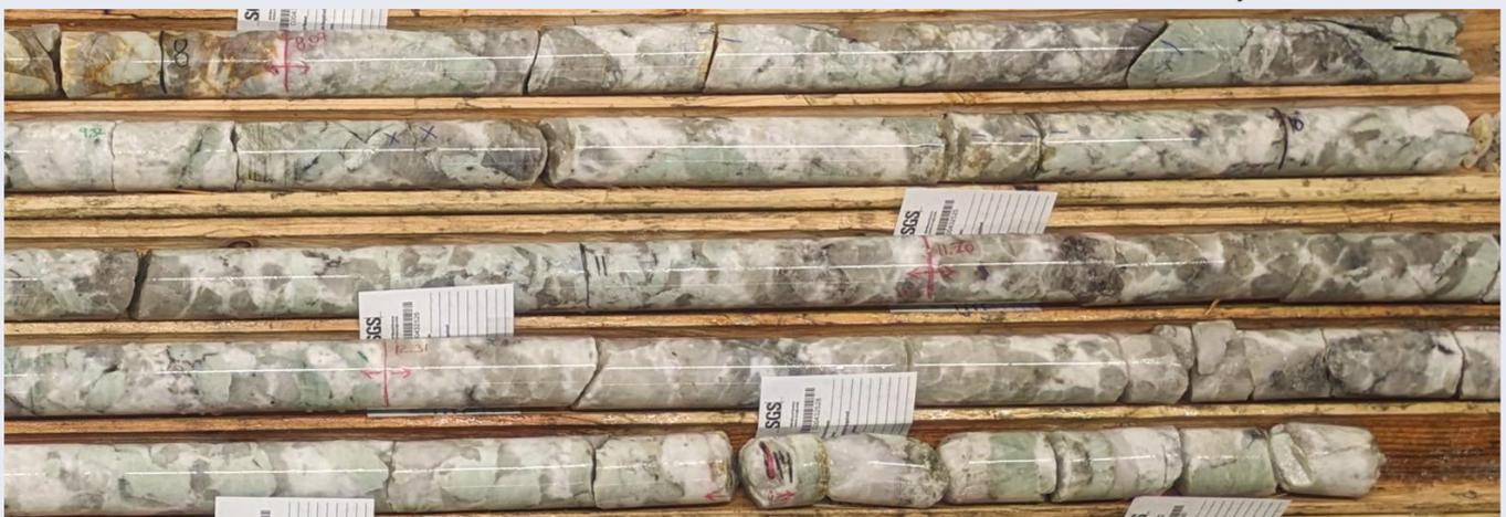
**Appendix Image 6: Trieste Lithium Project – Zoomed in core photo of Spodumene crystals drillhole TR24-002.**
