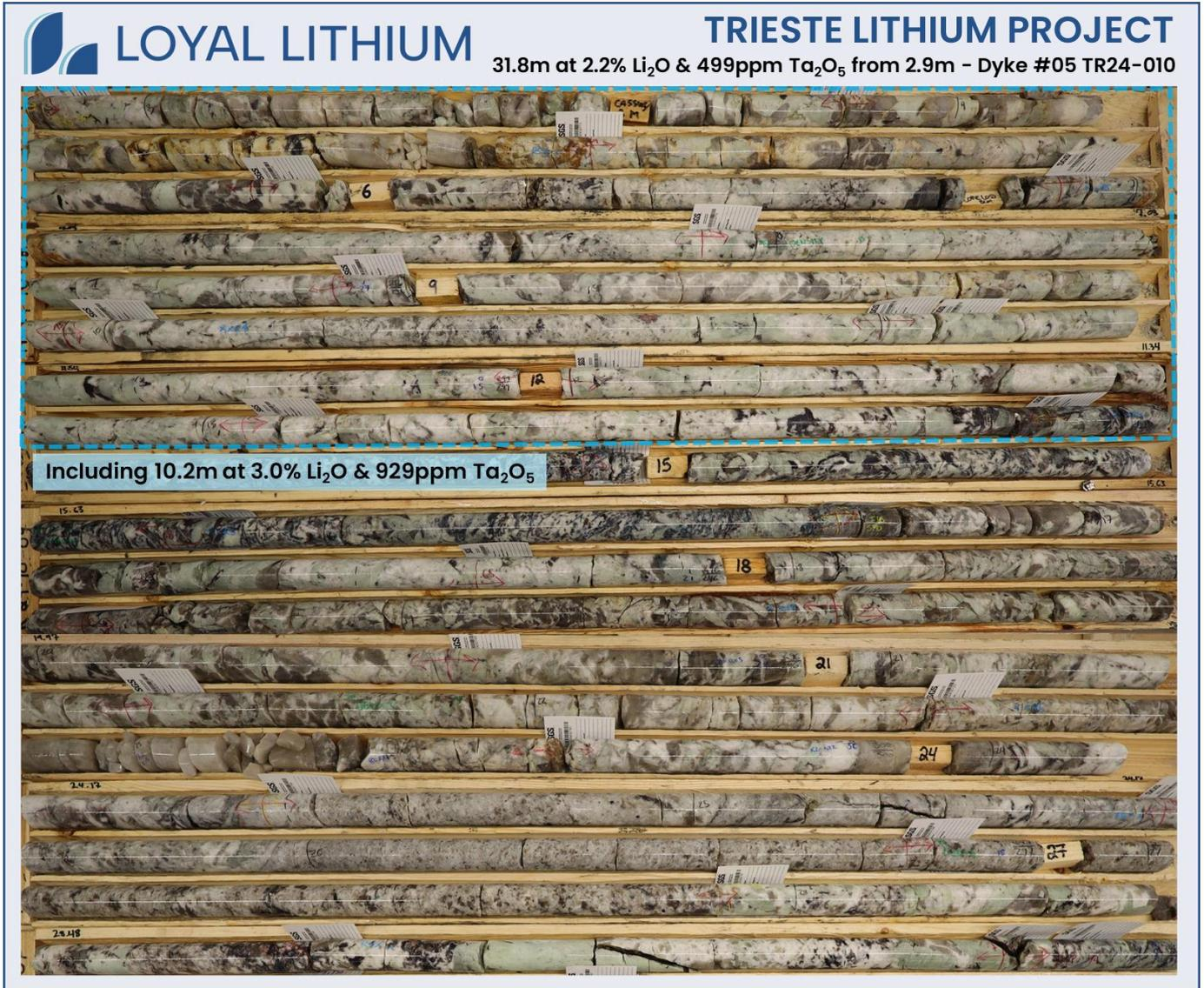
Appendix Image 3: Trieste Lithium Project - Dyke #05 core photo of Spodumene crystals drillhole TR24-010.
