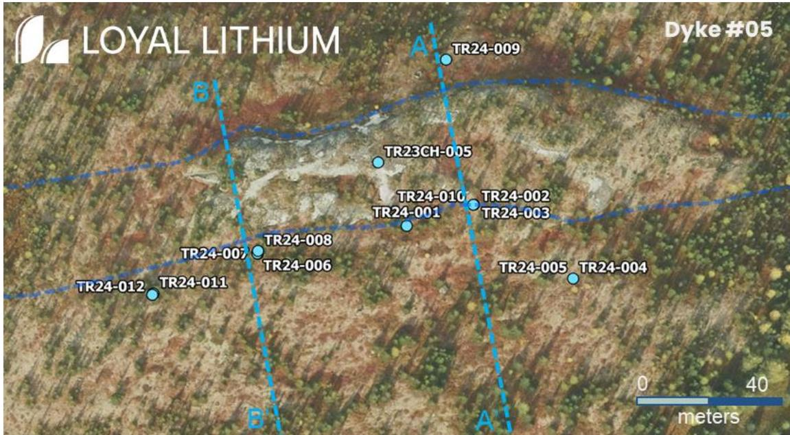
Appendix Image 1: Trieste Lithium Project - Dyke #05 plan showing drillhole locations and cross section lines.
