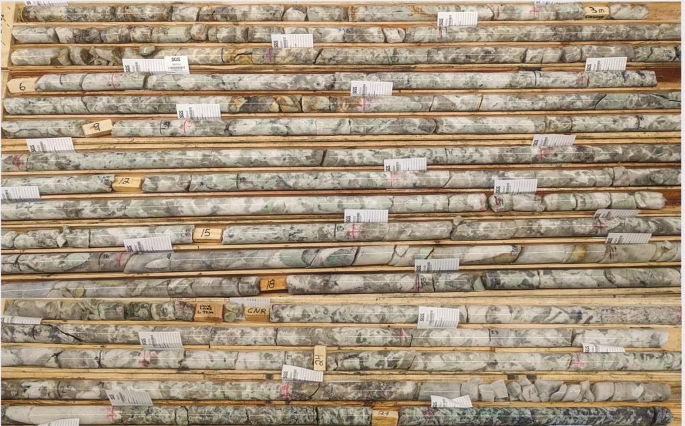
**Appendix Image 5: Trieste Lithium Project – Zoomed in core photo of Spodumene crystals drillhole TR24-002.**
