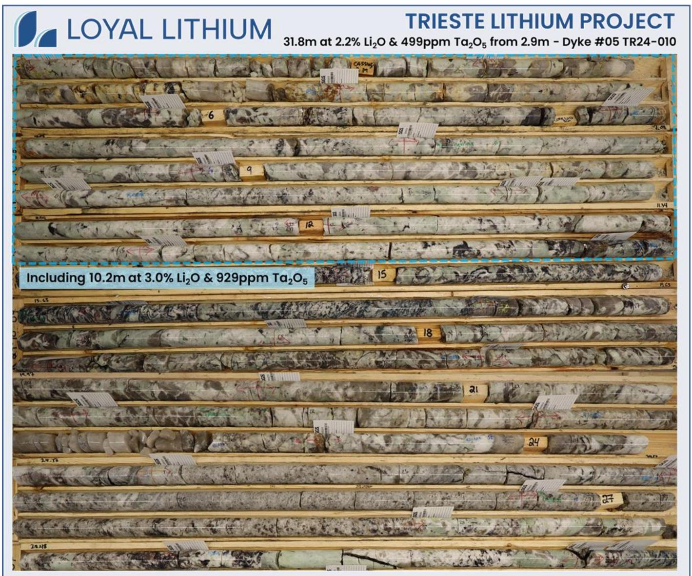
**Image 1: Trieste Lithium Project: Dyke #05 TR24-010 drill core showing significant spodumene mineralisation.**
