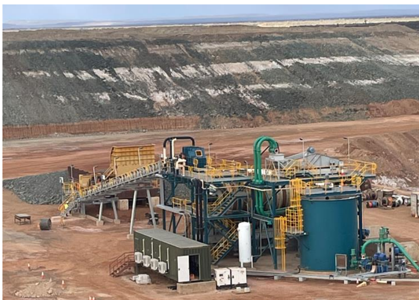
Figure 4: Wiltails feed system to CIL plant (TSF Western Cell in the background)
