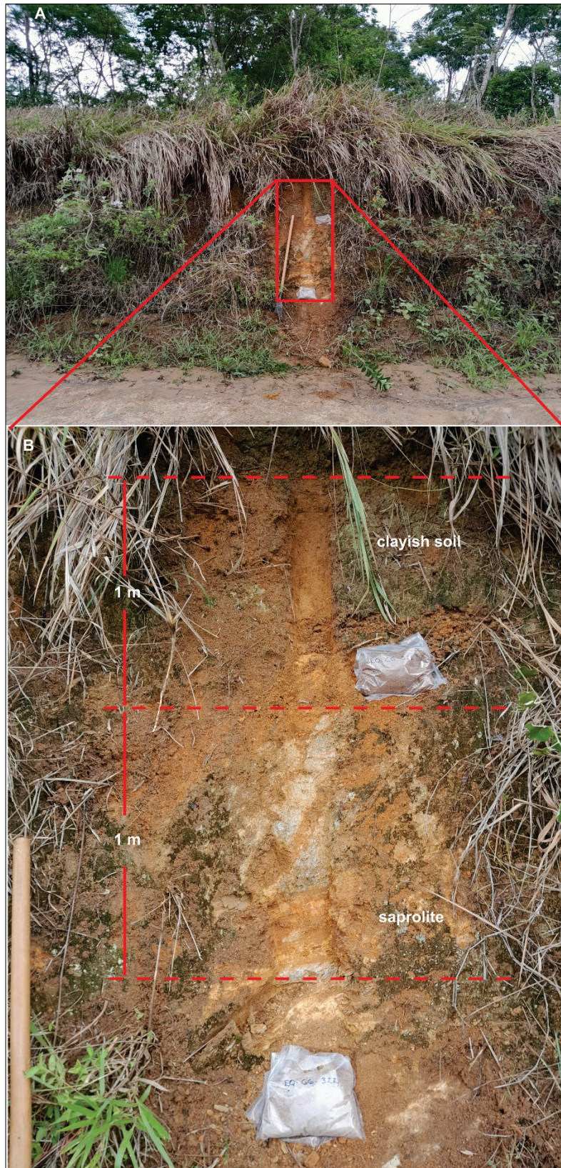
Figure 3: A) Outcrop in road cut with clayish soil (top) and saprolite (bottom) in anomalous region. B) Channel sampling detail.
