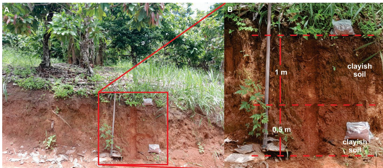
Figure 9: A) Road cut with clayish soil in anomalous region. B) Channel sampling detail.
