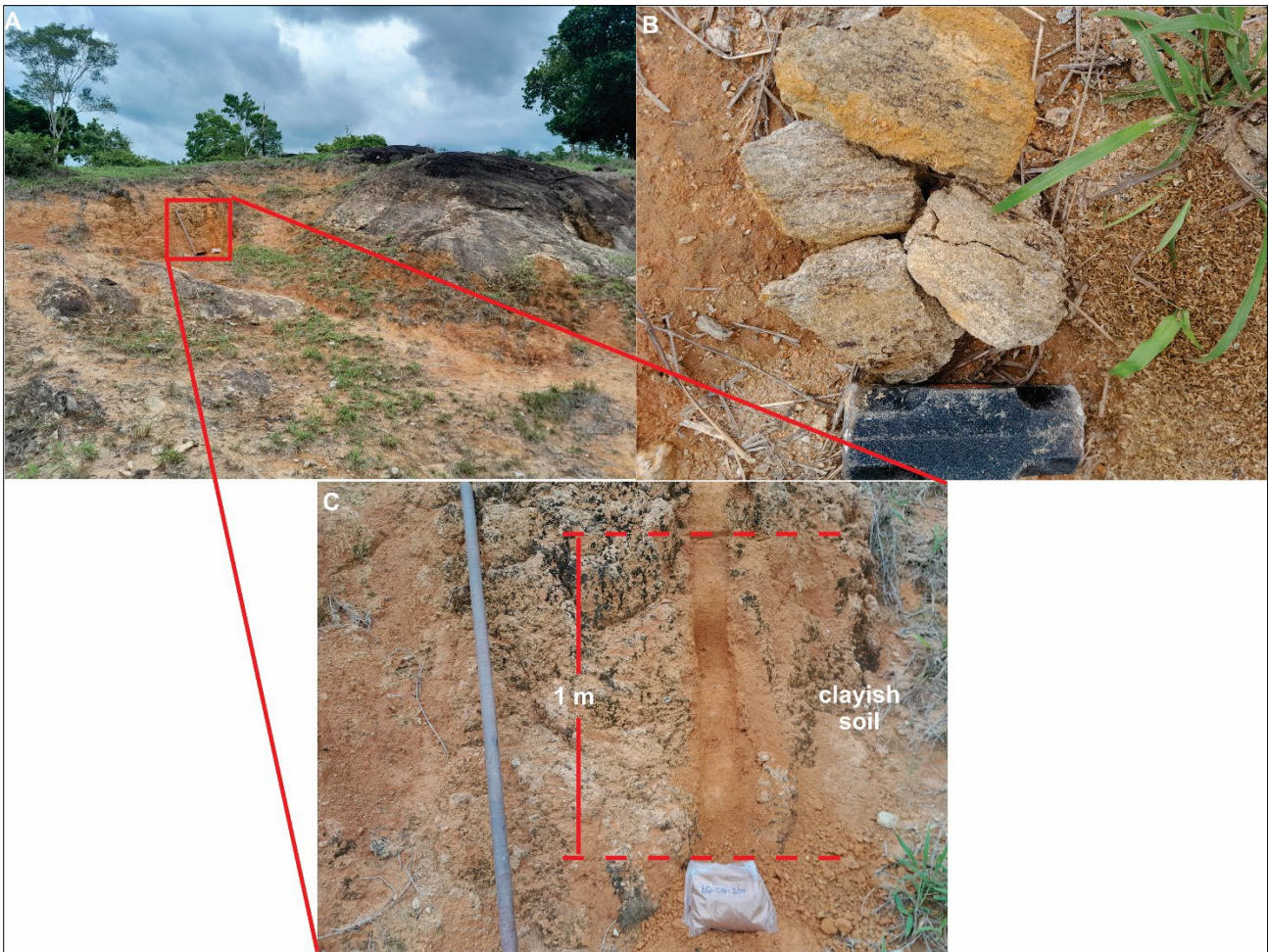
Figure 2: A) Leucogranite ortogneiss outcrop in anomalous region. B) Leucogranite ortogneiss detail. C) Clayish soil sampling.
