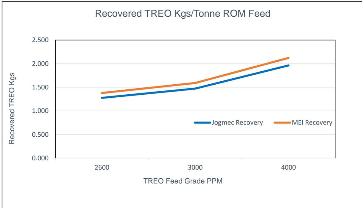
**Figure 6:** Recovered kilograms TREO per tonne ROM feed. New results significantly impact increased REE production rates.
