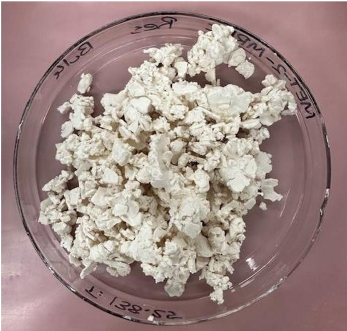
*Figure 3: Wet MREC after re-pulp and displacement wash.*
