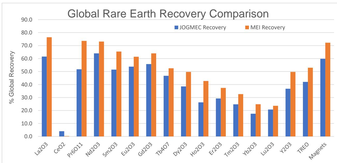
*Figure 5: Capaõ do Mel composite sample recovery comparison between historic and new test work.*
