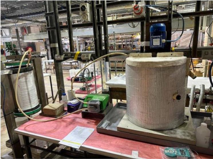
*Figure 1: MREC precipitation tank and setup at ANSTO.*
