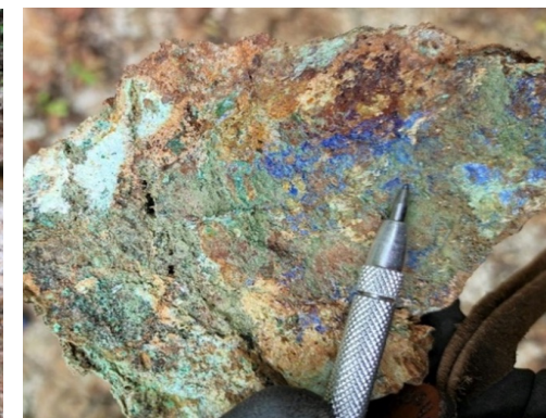
Copper Ridge hand specimen with Cu oxides
