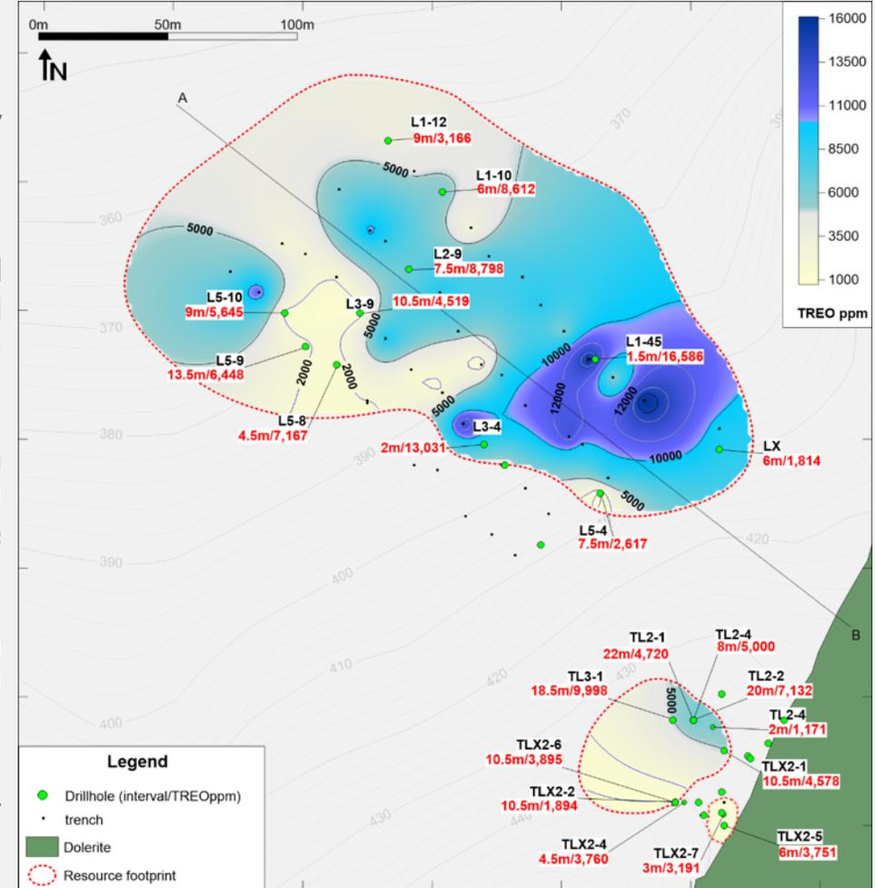
Drillhole Location Map on Trench Sampling TREO Contours
