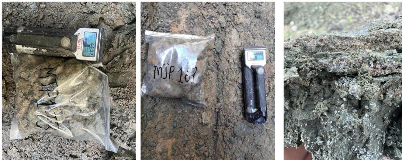
**Figure 2. Photos of the samples collected in pits 167 and 173 and high CPS readings**
