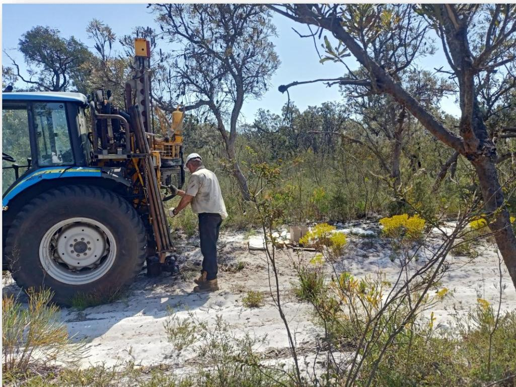
*Figure 2: Vacuum drilling at Muchea*
