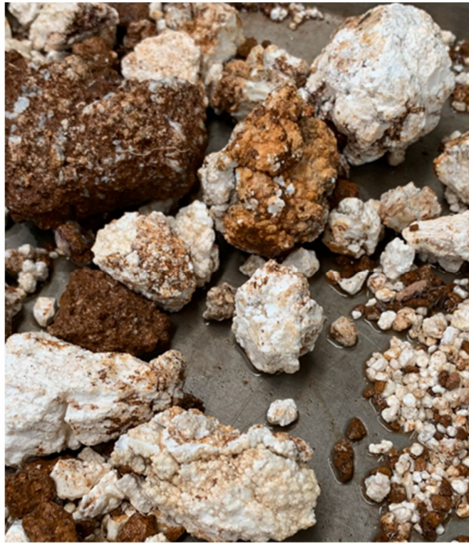
Figure 3: Coarse Material containing calcite, magnesite and gibbsite.
