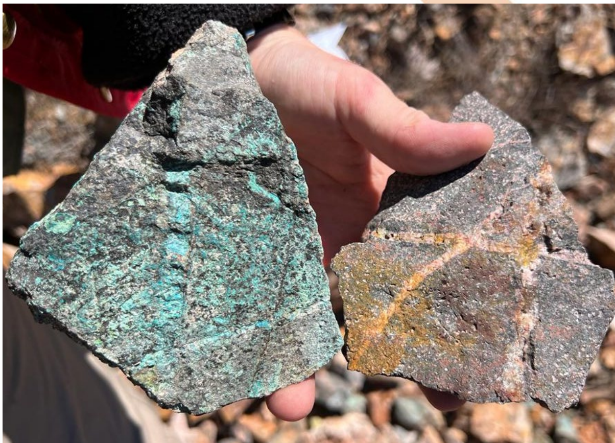
Figure 1: Sun Devil Prospect; blue-green secondary copper minerals, likely a complex mixture of chrysocolla, malachite & turquoise, coat a fracture which exposes a vein stockwork that overprints a pre-mineral brecciated meta-granitoid. Boxworks (vugs) and dark spots containing iron & manganese oxides are likely remnants of disseminated primary sulphides which have been leached by intense oxidation / weathering.
