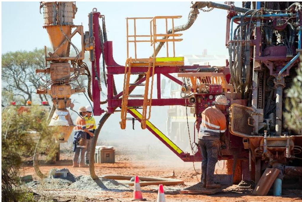
Figure 2: RC drilling at the Gifford Creek Carbonatite.
