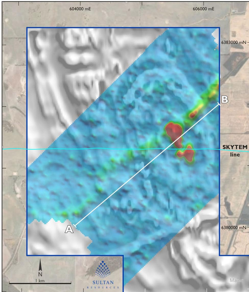
**Figure 2: Channel 34Z EM response image overlaying greyscale aeromagnetics from Sultan 2017 survey. Original SKYTEM line denoted by light blue flight line. Section Line A -B for Figure 3 below highlighted in white. Flight lines are 100m spacing.**
