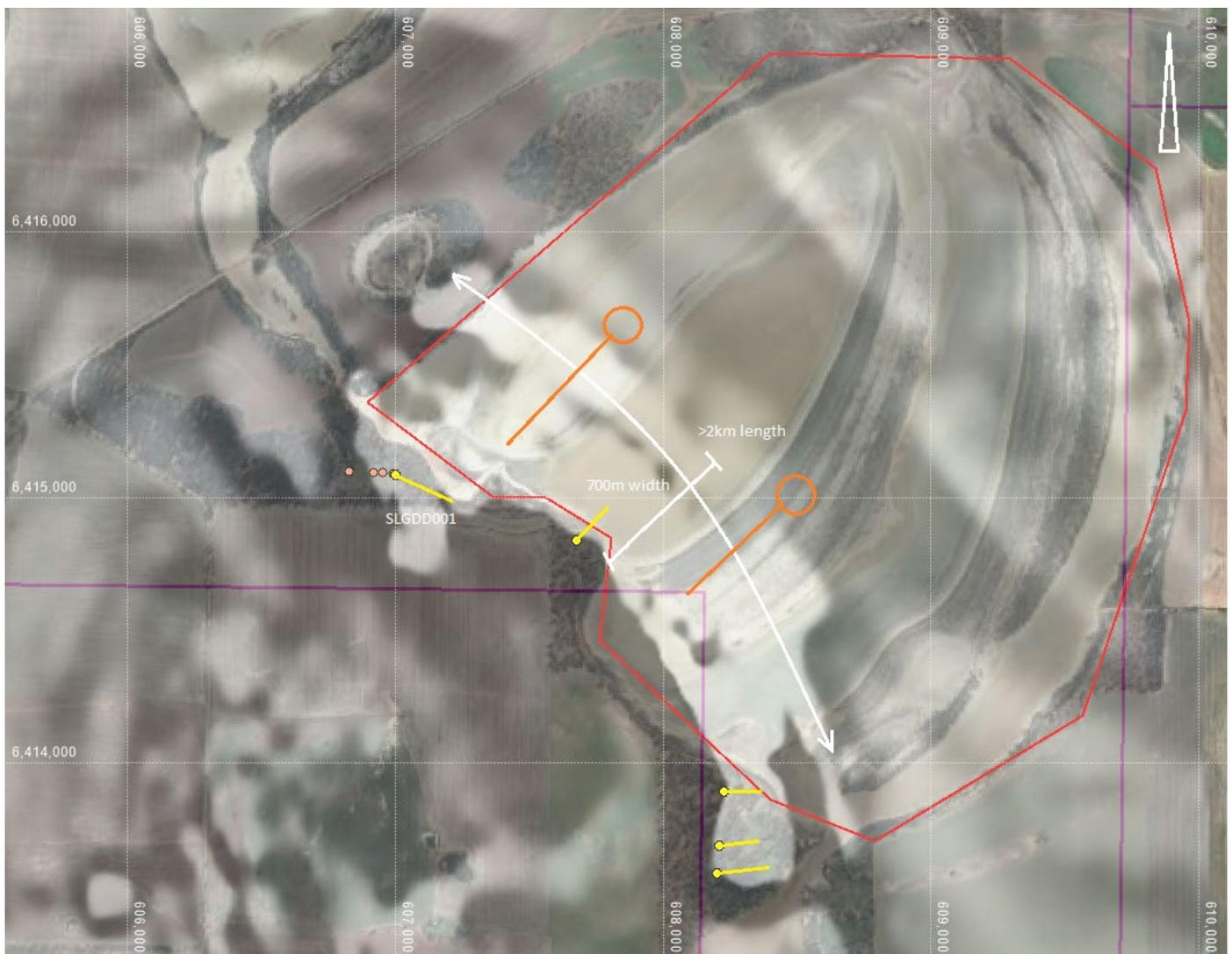
Figure 6: Plan view of 1VD magnetic signature representing the ultramafic sequence overlain by aerial photography highlighting the salt lake, with Reserve 18455 (Lot 225568) highlighted in red. Sultan’s 2022 aircore collars are marked in orange, and previous diamond drilling traces in yellow, with recent SLGDD001 named. Orange circles and traces indicate provisional drilling collar positions to test the layered intrusion from the salt lake surface.
