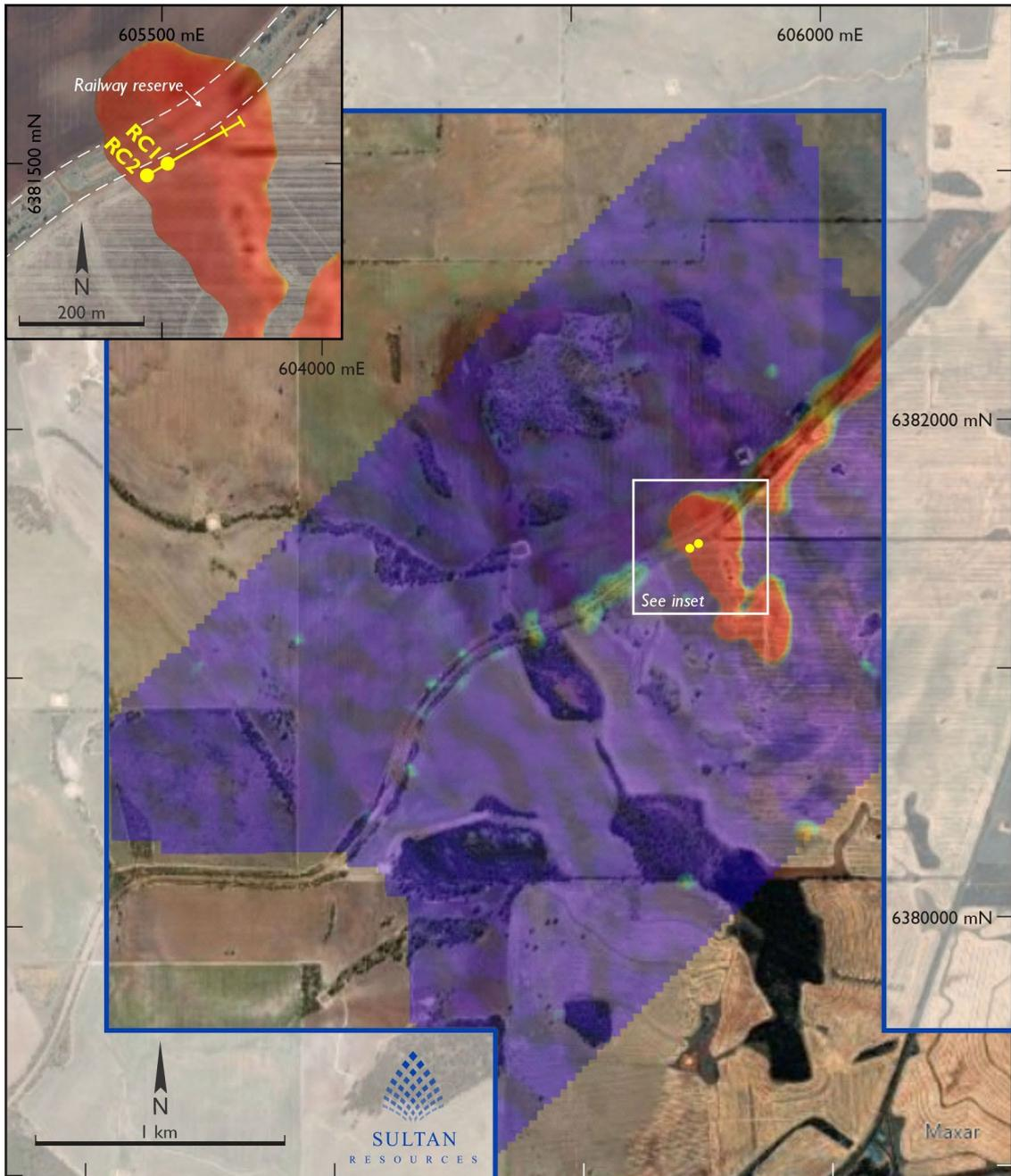
**Figure 1: Channel 24Z EM response image overlain on aerial photography, with tenement E70/5082 highlighted. EM data also indicates the position of the Tier3 Jitarning-Kulin rail line, closed since 2013. Initial planned 2 hole RC drill traverse highlighted in inset.**
