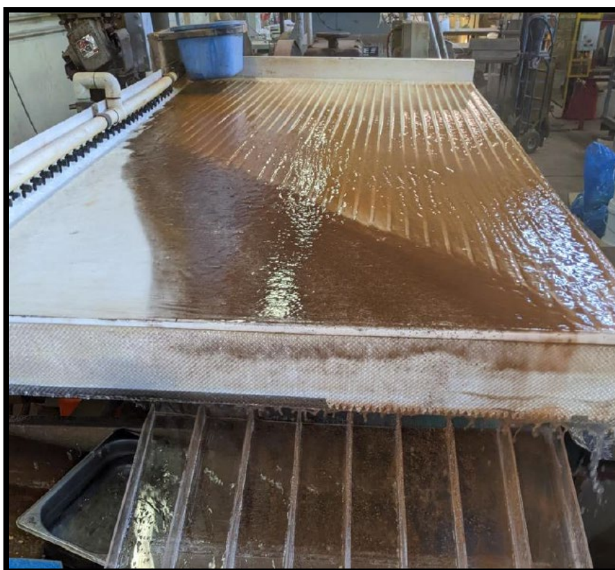
Figure 2: Laboratory Size Wilfley Table (View from Discharge End)
