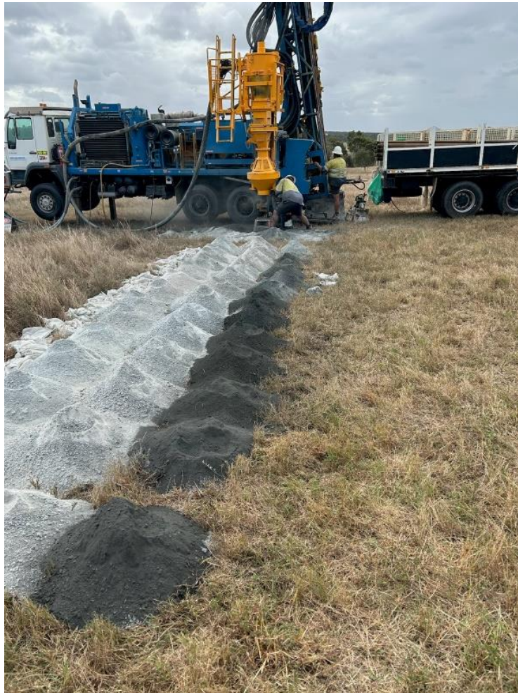
Figure 4: Black sulphide recovery from hole ARRC001 114m downhole with pale porphyry on left.
