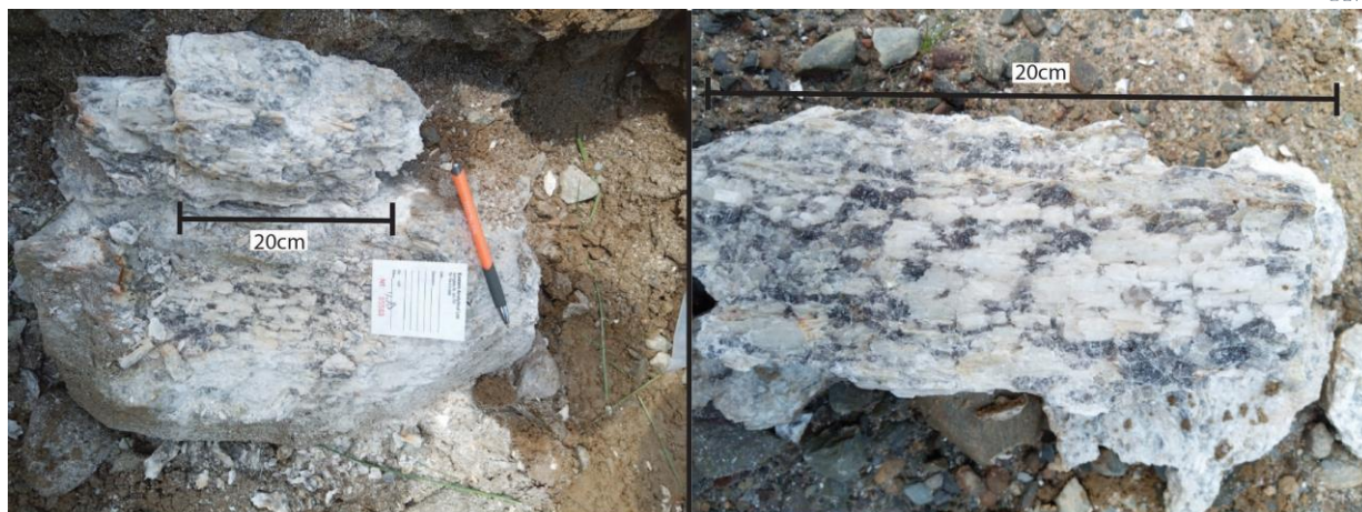
Photo 2- Boulder containing abundant Spodumene with quartz Occurrence 2 (Sample 85569)
