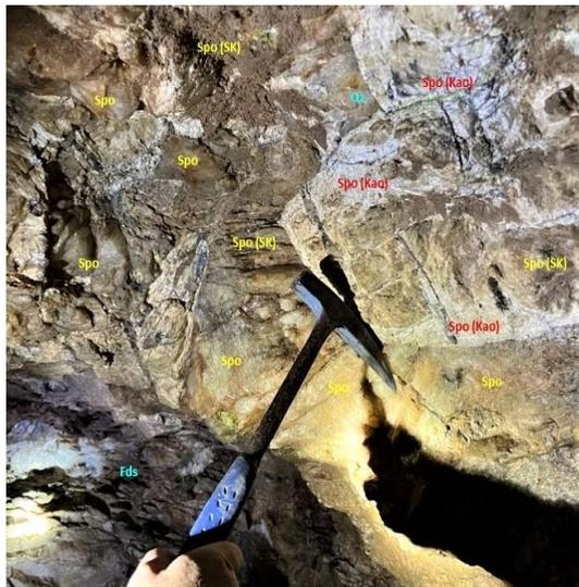
Typical of spodumene crystals within Spodumene Zone in Jaime Linopolis Sitio do Estevinho underground mine. Massive fresh spodumene (Spo) . White domains are partially kaolinized spodumene along fractures (Spo Kao). Spodumene with skeletal/corroded texture (Spo SK).
