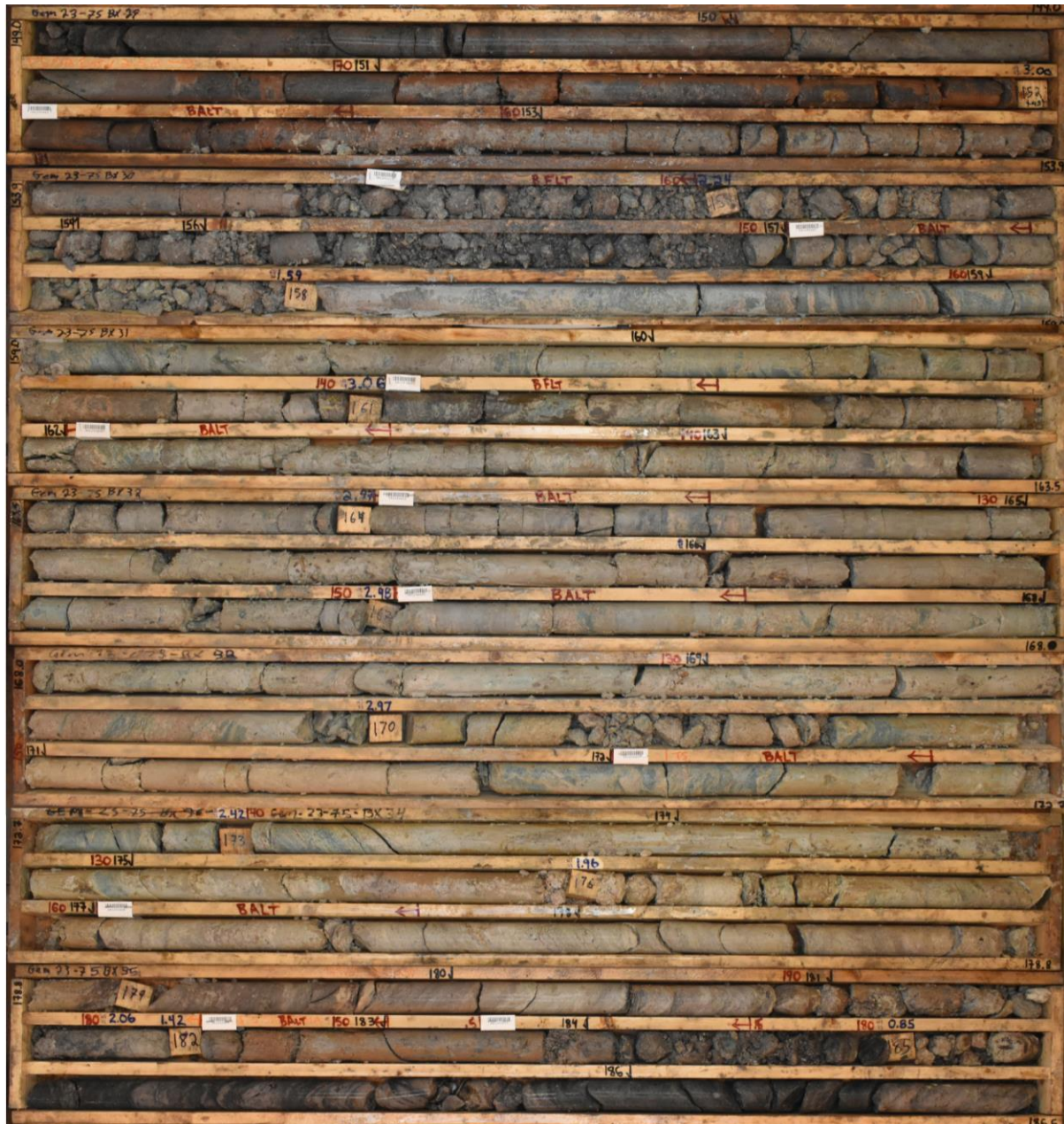
Figure 3: Strong brittle faulting with intense hydrothermal alteration in GEM23-075
