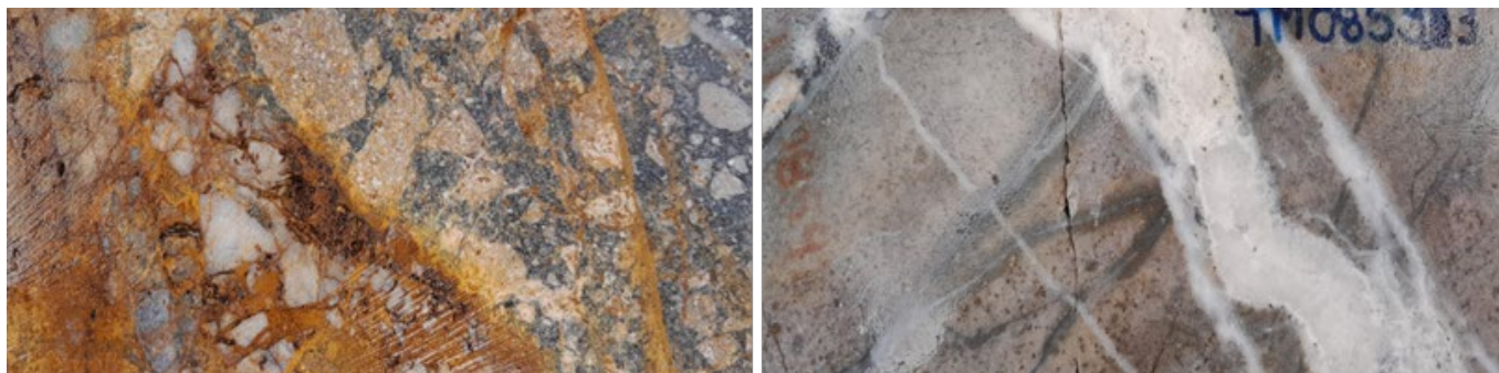
Plate 1. Resbolosa Vein Target. Left: CVDD23-106. Brecciated quartz vein with oxide filling between the clasts, cutting the tourmaline breccia, there is also a second phase of transparent quartz veinlets with trace mineralisation of pyrite, sphalerite. Right: CVD008. Greyish quartz veinlets with mineralisation of pyrite, galena, sphalerite, traces of arsenopyrite, cut by a veinlet of white quartz with traces of pyrite.
