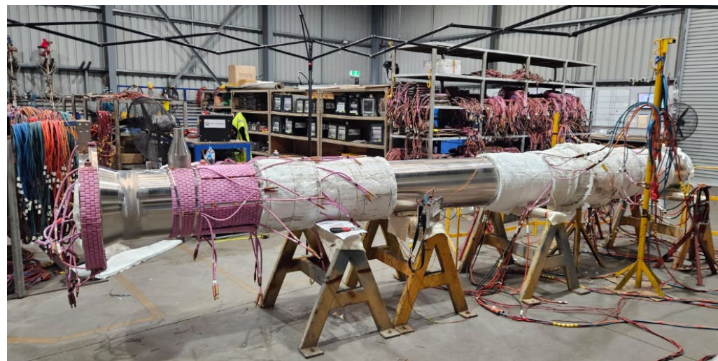
Reactor successfully heat-treated and preparing for final assembly and machining
