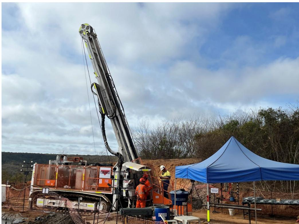
Figure 7: CS3001 drill rig, one of the two metallurgical drill rigs currently on site, drilling SAMT002.
