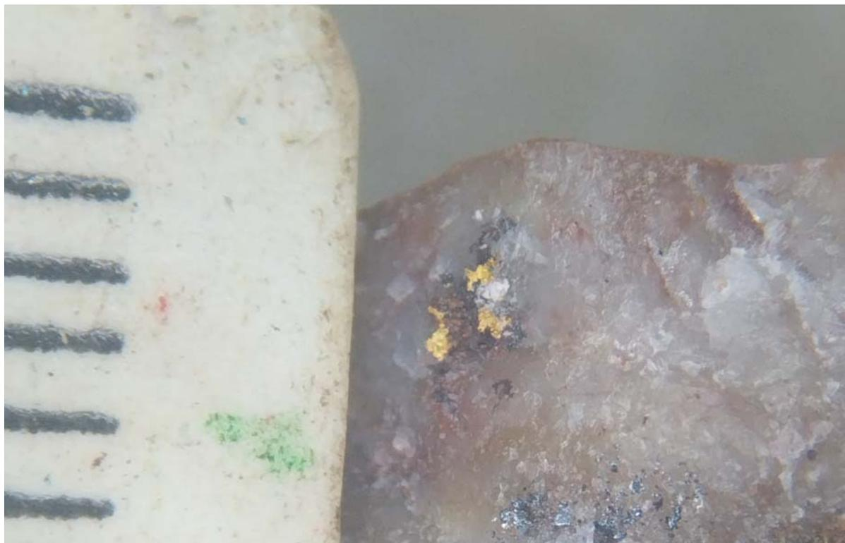
Figure 1 Visible gold from sample HYPSS2310 taken from the Brokenwood prospect – scale to left is 1mm (See Table 2 for location of sample).
