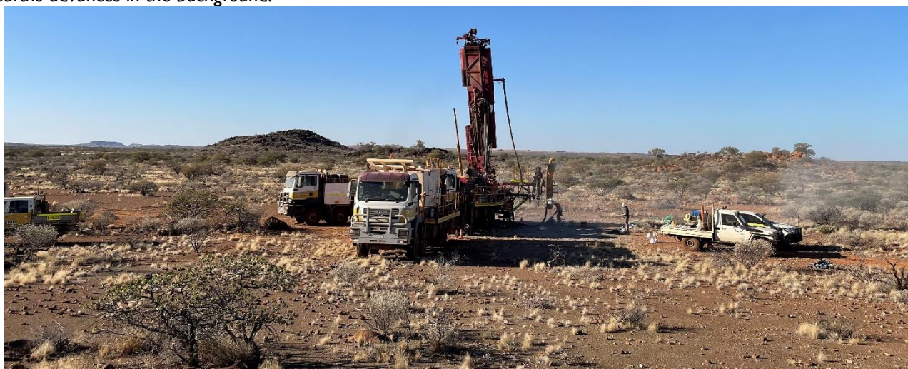
Figure 1: Photo of the RC rig drilling at Bookathanna North.
