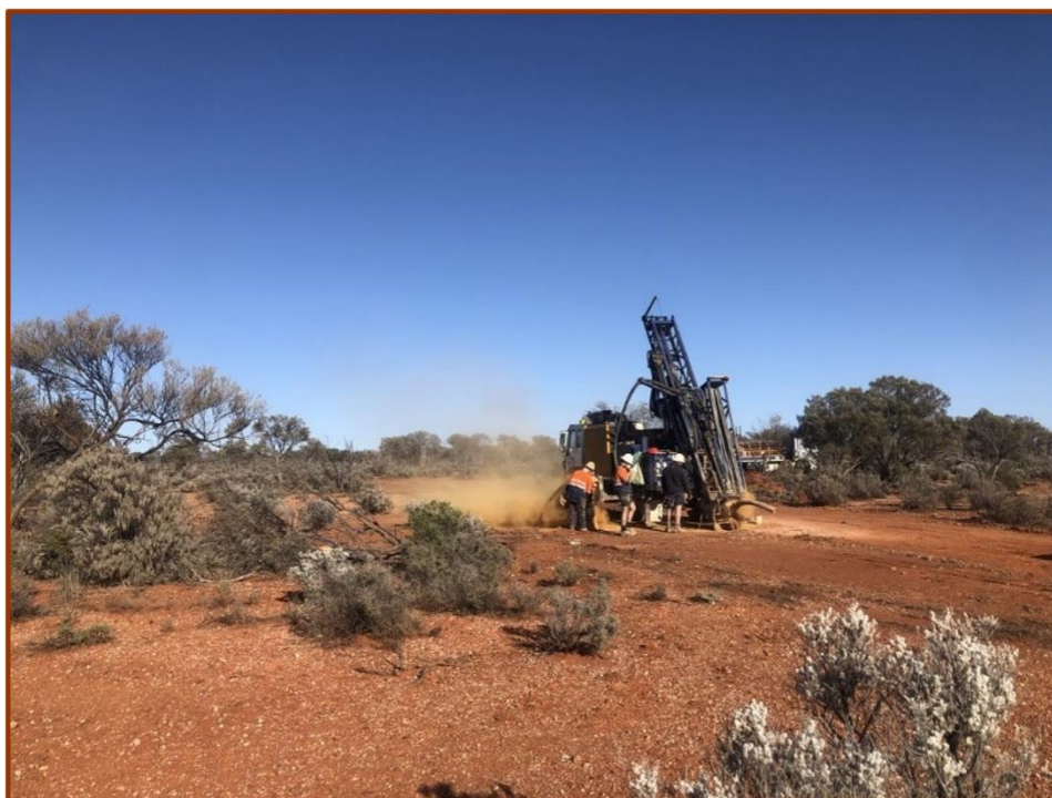
Figure 3 – Air-core Drilling at Edjudina
