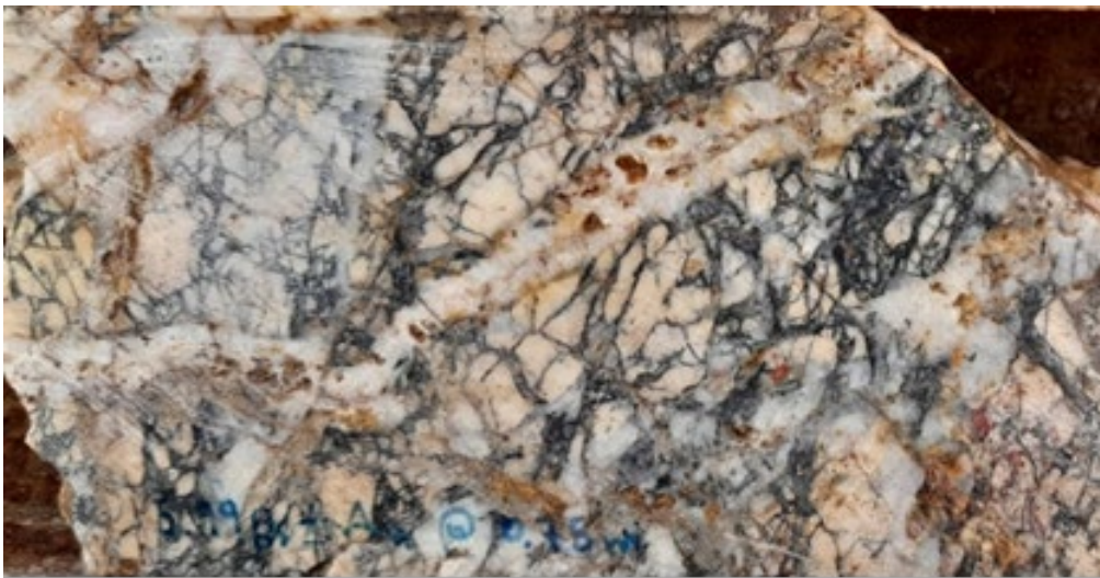
Plate 1.05DDH04:22m. White quartz vein, brecciated, filled with Ag, and cut by later more transparent quartz veinlet.
