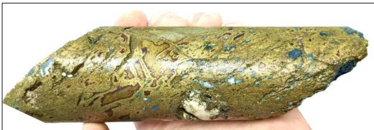
Figure 1: Chalcopyrite in LTDD22074 (101.1 -101.25m) from a broader interval grading 3.9m @ 8.30% Cu from 99m.
