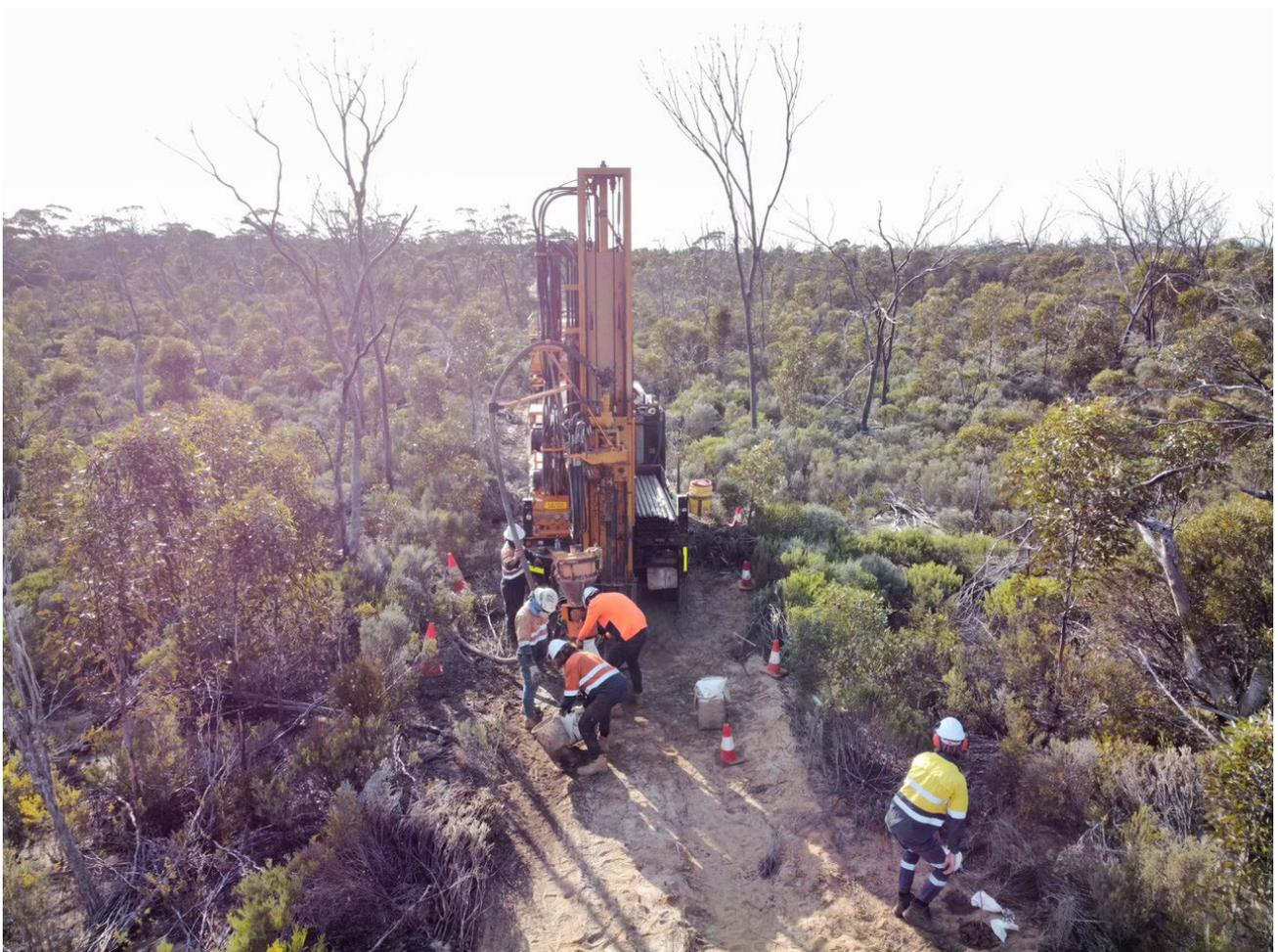
*Figure 1 – Air Core drilling rig in operation at Dingo Rocks.*
