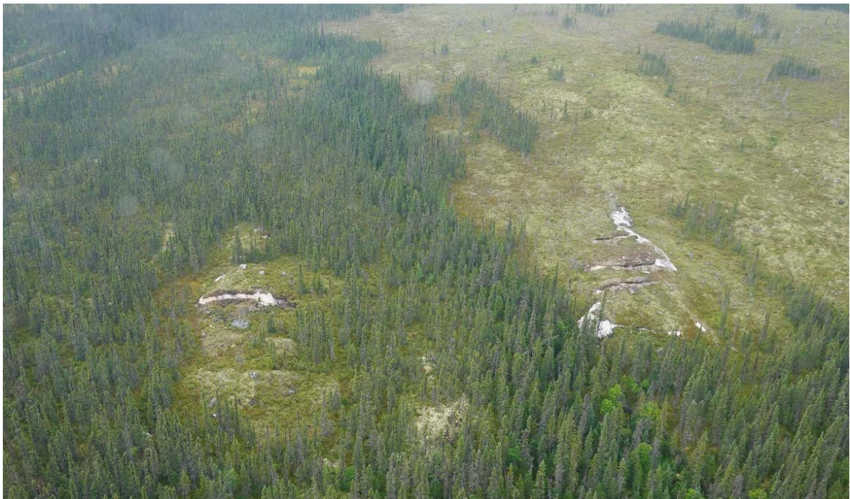
Figure 1. Aerial view at Ruby Hill West looking to the west of the RHW-1 (to the right) and RHW-2 (to the left) pegmatites and 2023 trenching. The RHW-2 trench is 30m long with the collar from RHW22-06 located near the southern end of the trench.
