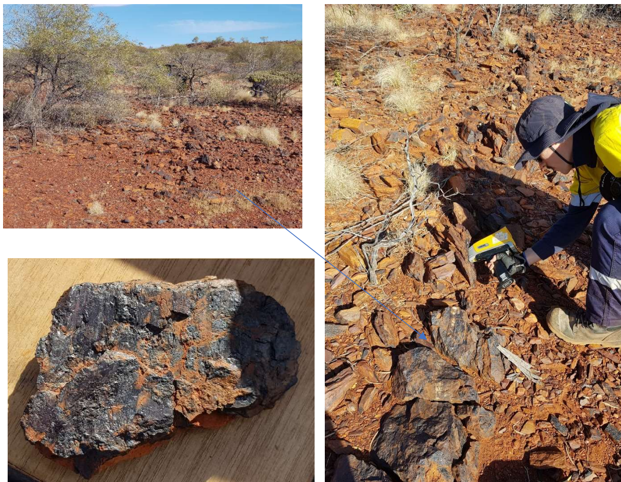
Figure 4. Anomalous REE zones (identified from Portable XRF measurements) adjacent to subvertical N-S trending thin quartz veins associated with apparent dextral strike-slip faulting in E09/2422 (367,000mE, 7,373,020mN GDA94 Z50); wet chemical analyses are in progress.
