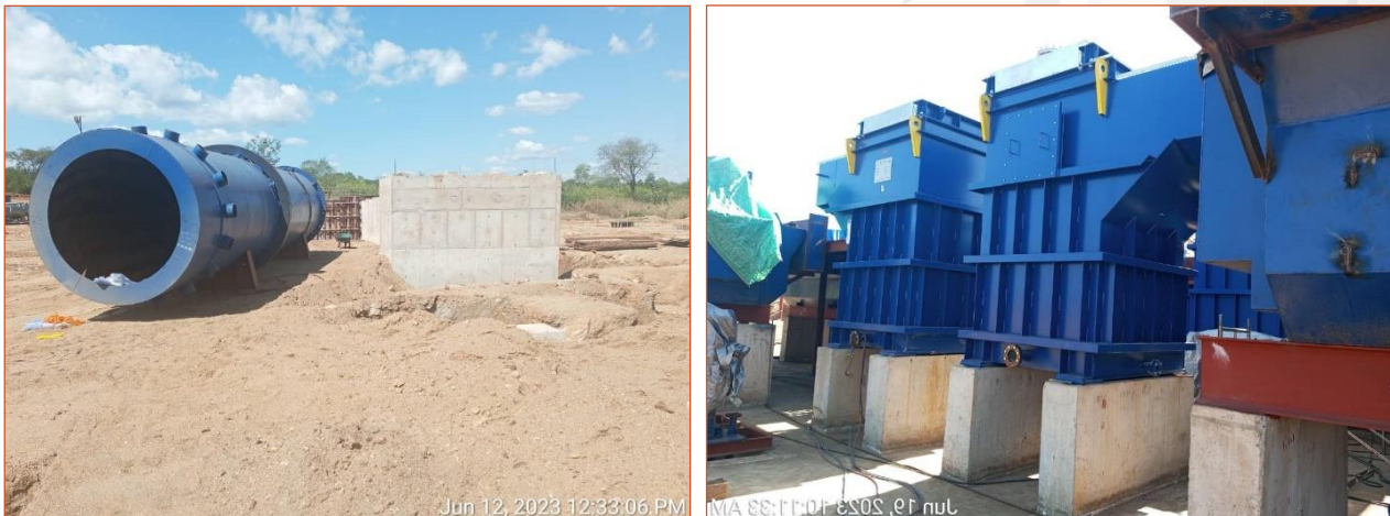
Figure 2: Two of the rotary driers on site (left) and the Attritioning mills installed on their plinths within the Concentration Building area (right).
