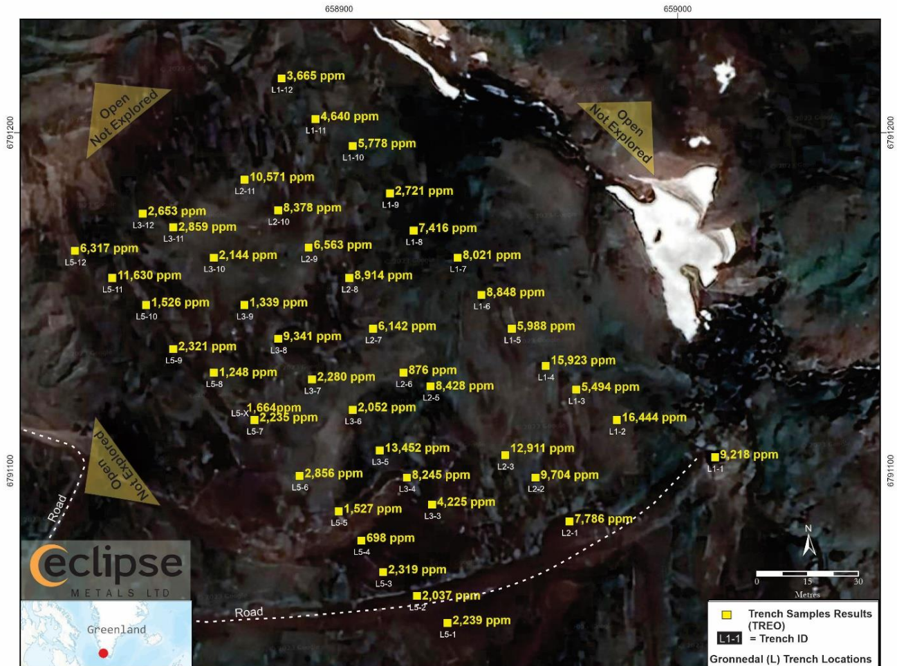
Figure 10. Grønnedal trench sample results in the lower section with REO mineralisation in all trenches. Note that, to date, only a small fraction of this prospect has been explored and that the system is open in all directions.
