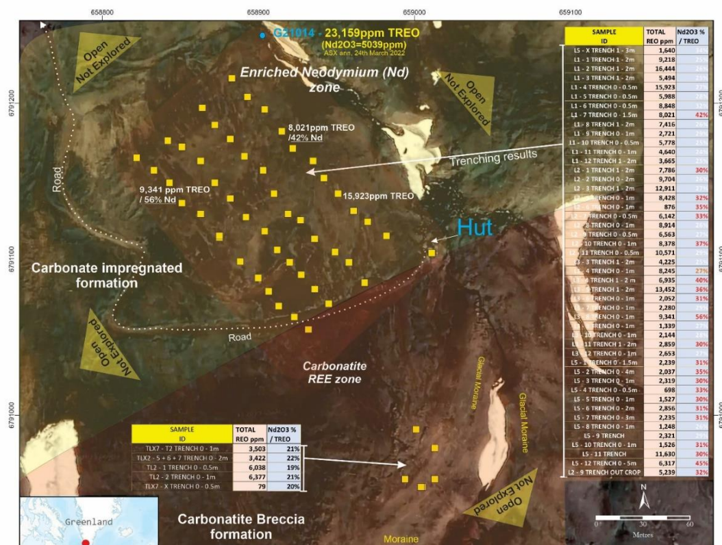
Figure 13: Conceptual overlapping styles of carbonate impregnated formations and carbonatite breccia formation within the carbonatite REE mineralisation
