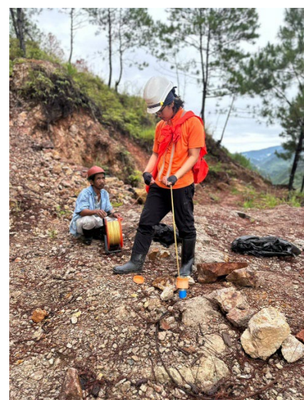
Data retrieval from vibrating wire piezometers (left) and water level reading of completed drill holes (right)
