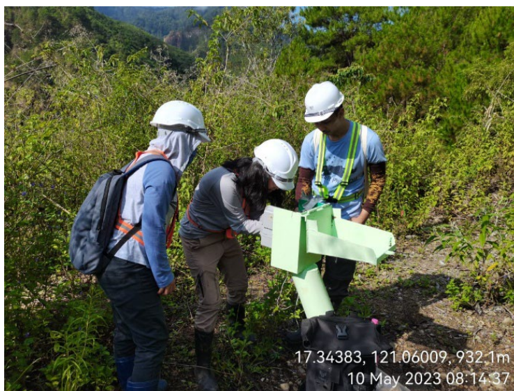
Data retrieval from vibrating wire piezometers (left) and water level reading of completed drill holes (right)
